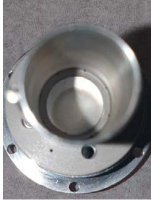
Figure 4.1: Photograph of the rear part of a Faraday cup exposed to the ion beam. The circle distribution is defined by the probe aperture diameter.
