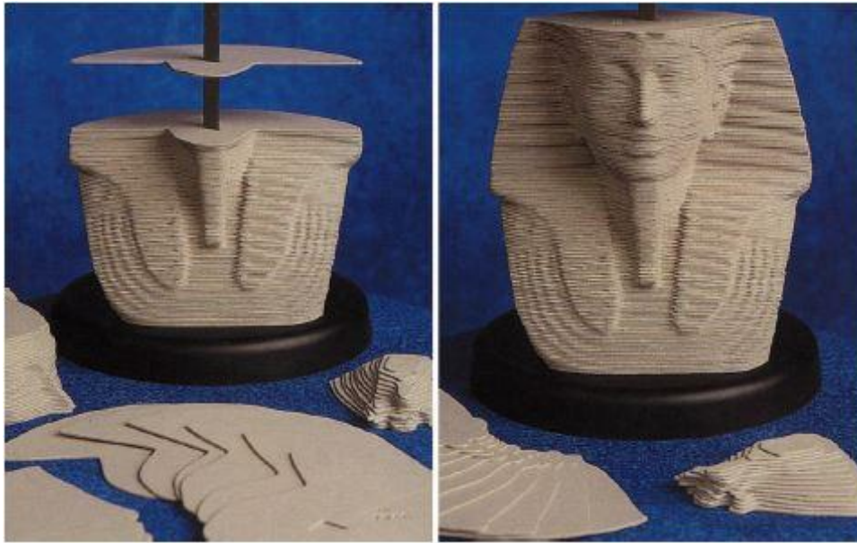
Figure 1. Principle of AM: A 3D-object is generated via staggered layers. [16]
