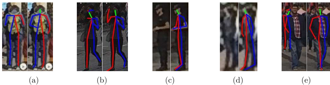
Figure 5.2: Comparison of poses generated by OpenPose and HRNet: For each image pair, the left image depicts the pose generated by OpenPose and the right image the pose generated by HRNet.
