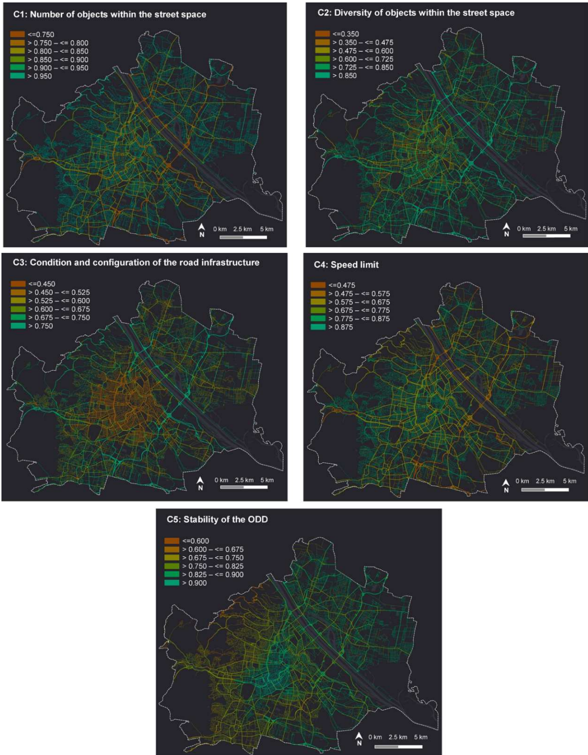
Fig. 3. Assessment of the automated drivability for the city of Vienna based on the values of ADX (above) and assessment for the five different components (below).
