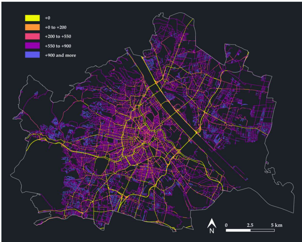
Figure 7. Possible increase of number of vehicles at peak hour until completely not compatible in the reference scenario.
