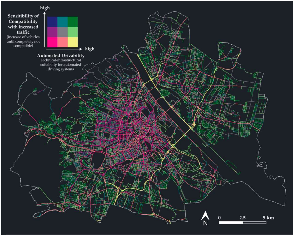
Figure 8. Overlap of the assessment of the sensibility of compatibility with increased traffic (in the reference scenario) and the assessment of the automated drivability.
