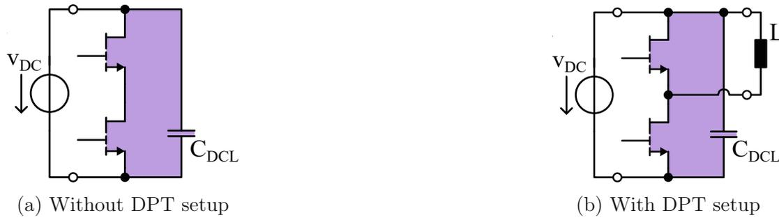
Figure 3.13.: Simplified schematic of a half-bridge with commutation loop (purple area)
