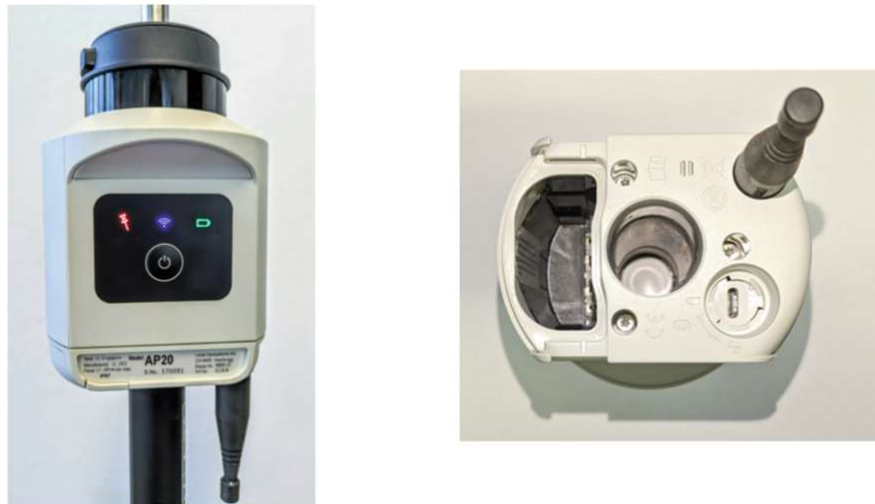
Figure 3.3: Left: AP20 Autopole Interface with LED icons Right: Battery compartment with USB-C interface and antenna
