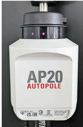
Figure 3.4: Target ID: LED strip showing unique signature
