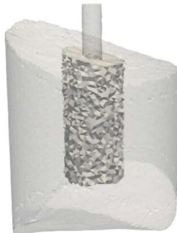
Figure 2.19: Cylindrical VOI of the hFE model approach
