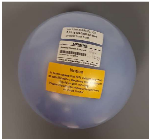
Figure 2.3: Spherical Phantom 18 blue from Siemens used for all phantom measurements in this thesis.
