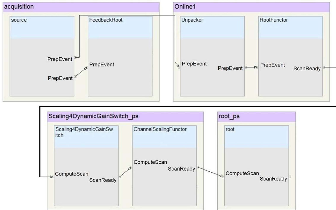
Figure 2.13: Diagram of the default ICE pipeline for the CRT reconstruction showing its pipe services and functors .
