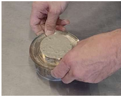
(a) Filled Slump-Flow Cone Just Before Lifting
