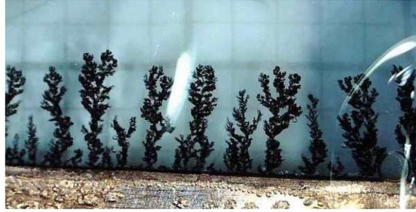
**FIGURE 2.8:** Exemplary image of dendrites grown from a  $\text{CuSO}_4$  electrolyte.
