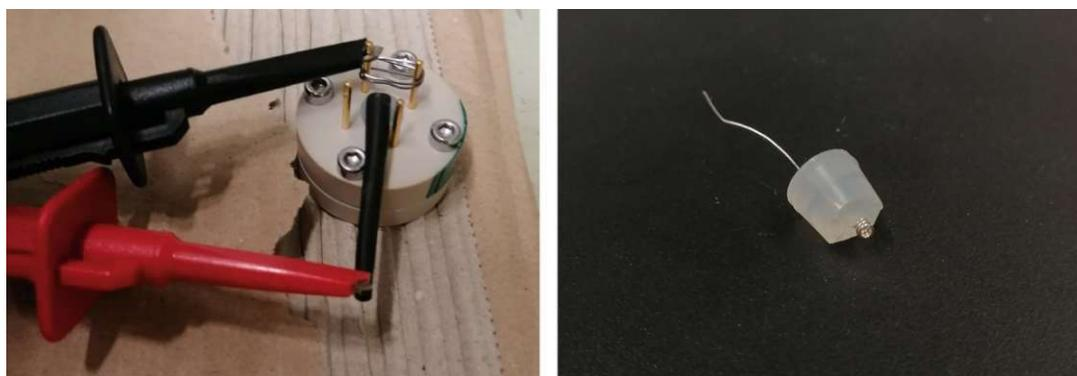
**FIGURE 3.7:** (left) Fully assembled ITC cell with contacted clamps. (right) Image of the rubber stopper with metal coil.
