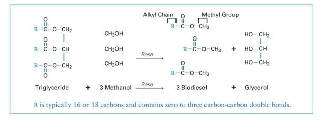
Figure 4: Scheme of transesterification of vegetable oil with methanol to biodiesel [60].
