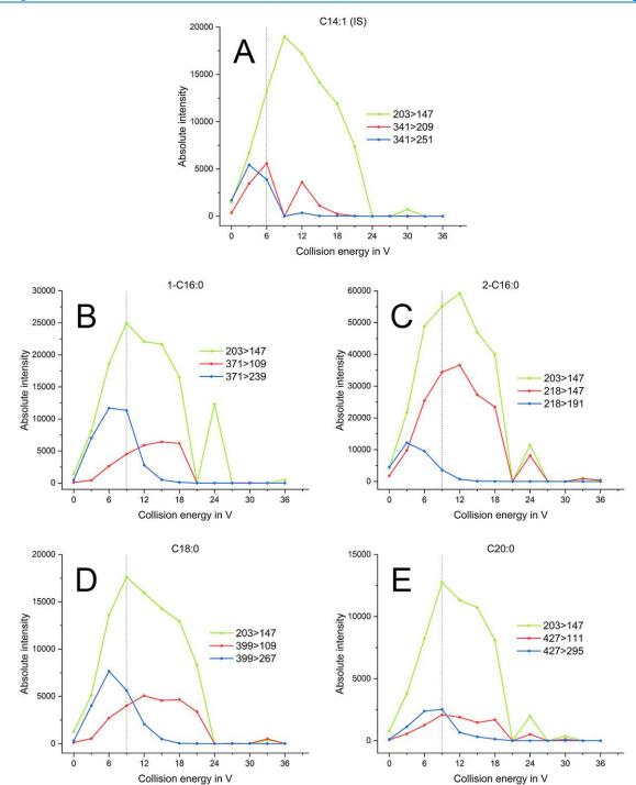
Figure 2. Intensities of the specific qualifier (blue and red lines) and quantifier ions  $(m/2\ 203 > 147, green lines)$  at different collision energies are shown for the IS C14:1 (A), the single SMG standards 1-C16:0 (B), 2-C16:0 (C), C18:0 (D), and C20:0 (E). Dotted line marks the chosen collision energy at 6 V (A) or 9 V (B-E).
