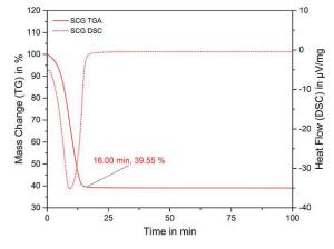
Figure 19. Drying rate of SCGs with TGA/DSC.
