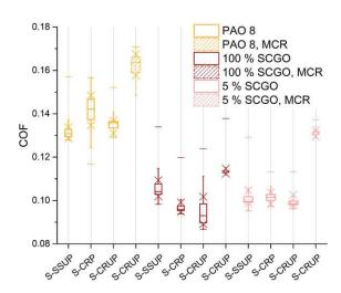
Figure 6. Box-and-whisker-plot of COF on different surfaces of nanotribometer and rheometer measurements. The box is giving the lower (25%) and upper (75%) quartile, whiskers are used to represent all samples lying within 1.5 times the interquartile range (IQR). Median line (thick horizontal line), quantiles  $Q_{0.1}$  and  $Q_{0.9}$  (cross), and maximum and minimum values (thin horizontal line) are displayed.
