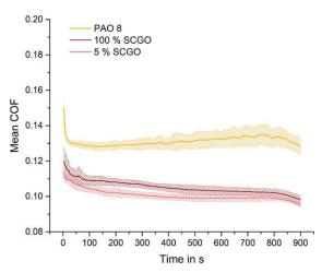
Figure 7. Friction values of nanotribometer experiments of different oils on unpolished S-SSUP given with standard deviation between data sets (n = 3).
