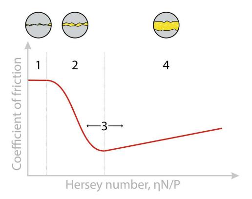
Figure 5: Schematic Stribeck curve showing 1. boundary lubrication, 2. mixed lubrication, 3. elastohydrodynamic lubrication, and 4. hydrodynamic lubrication. Adapted from [96].
