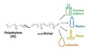
**Figure 4.** Conversion scheme of polyethylene to  $\alpha_i \omega$ -divinyl-oligomers and possible applications. With permission from (201).
