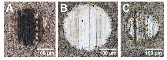
Figure 13. 2D-microscopic surface images of wear tracks after rheometer experiments using (A) PAO 8, (B) 100% SCGO, and (C) 5% SCGO in PAO 8 on unpolished S-CRUP samples.
