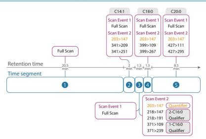
Figure 1. Scheme of time segments and scan events of C14:1, 1-C16:0, 2-C16:0, C18:0, and C20:0 showing full and MRM scans for the improved GC-MS/MS method. Ion transitions are displayed as m/z values, and quantifier ion transitions are highlighted in orange.
