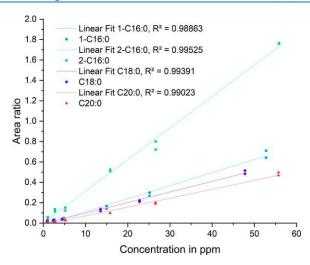
Figure 4. Calibration functions for 1-C16:0 (light blue), 2-C16:0 (green), C18:0 (violet), and C20:0 (red) at different concentration levels in CHCl<sub>3</sub>.
