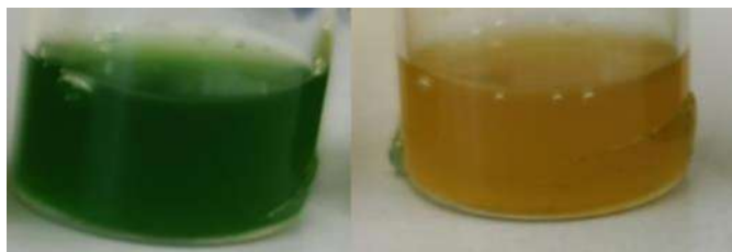
Figure 45 S. sp. PCC11901 fadA::PAD before (LEFT) and after (RIGHT) adding 10mM ferulic acid. Cells were incubated with 10 mM ferulic acid and converted into 4-vinyl guaiacol by the expressed enzyme PAD. The mixture was incubated for 24h at 39°C, 500 \mu\text{mol photons/s/m}^2 in a closed glass vial.
