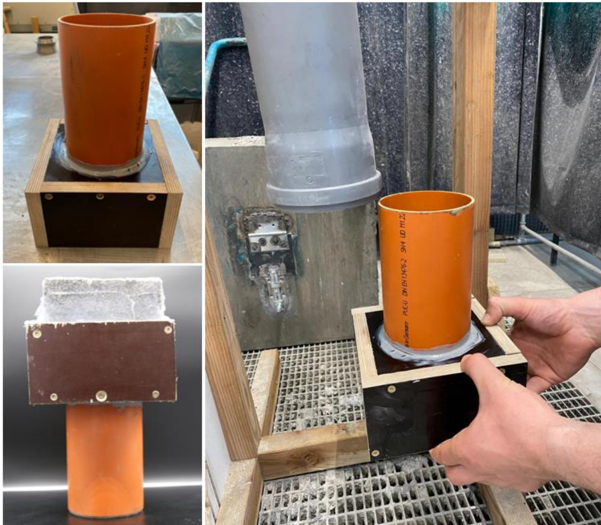
Fig. 3. 23. Setup for the measurement of water permeability
