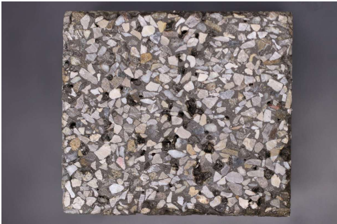
Fig. 4. 7. Sample with 40 % slurry quantity related to the aggregate mass.
