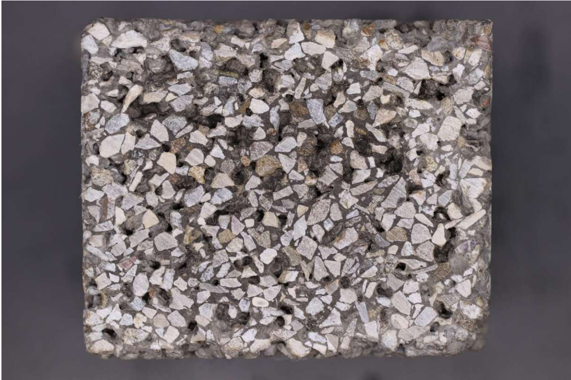
Fig. 4. 8. Sample with 35 % slurry quantity related to the aggregate mass.
