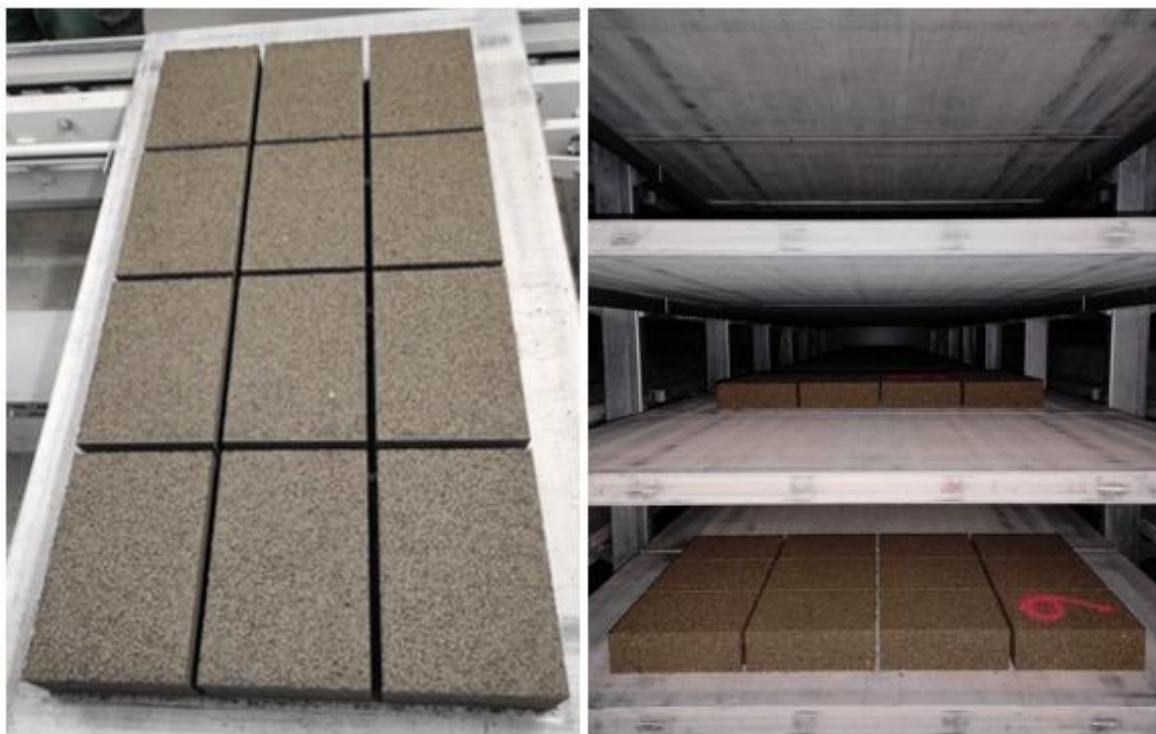
Fig. 2. 7. Water permeable pavers after vibrating and compaction process and drying chamber [7]
