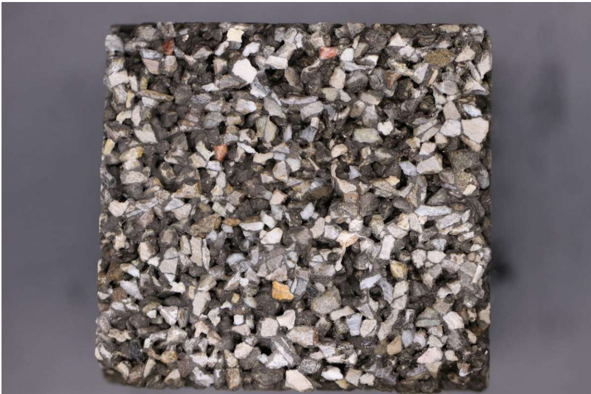
Fig. 4. 9. Sample with 28% slurry quantity related to the aggregate mass.
