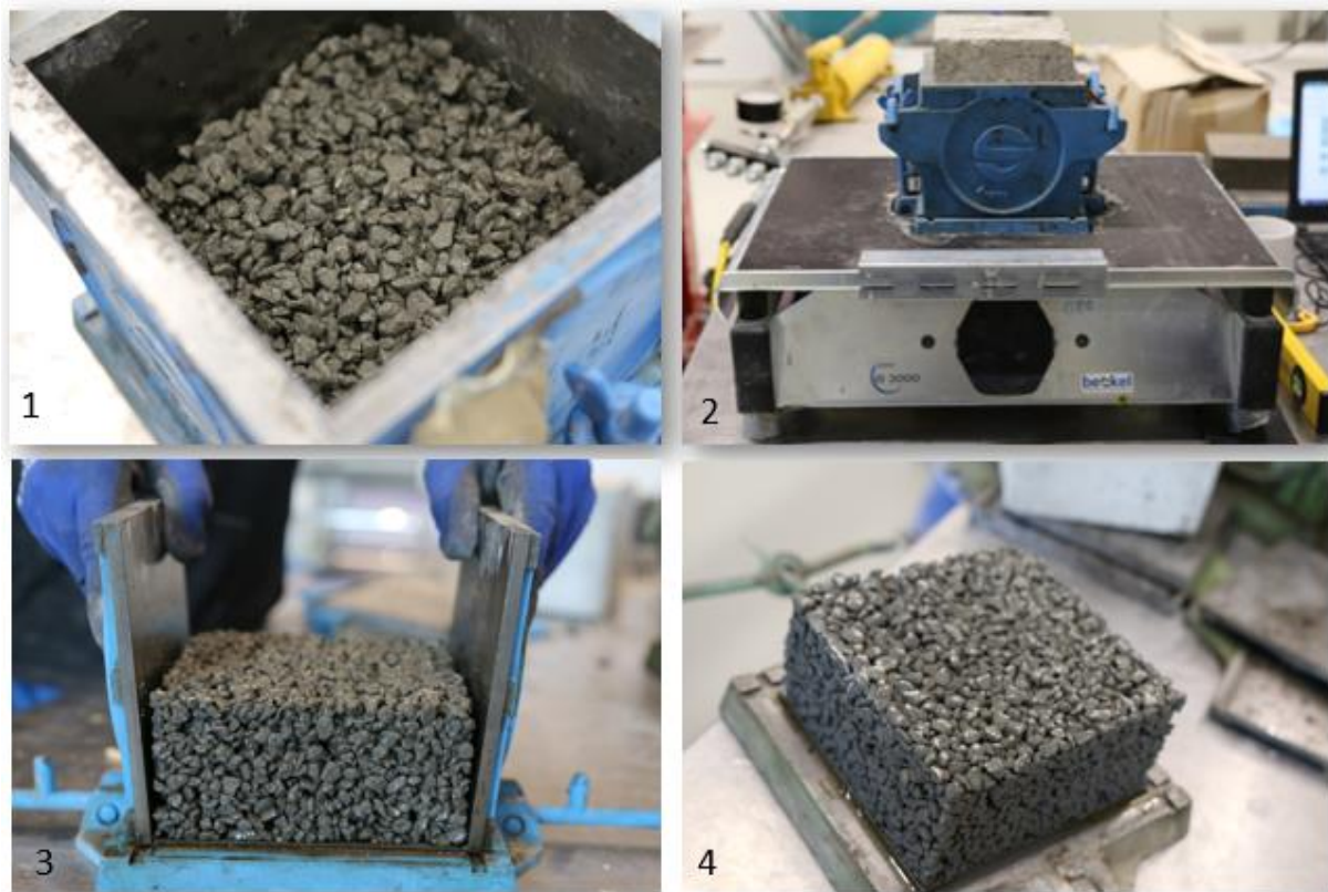
Fig. 3. 21. Vibration, compaction, and demolding processes
