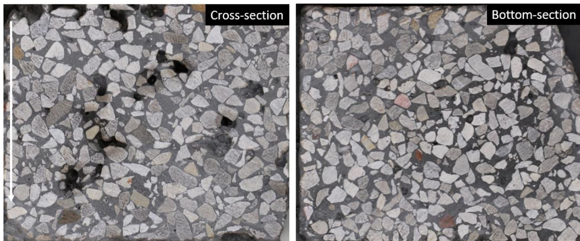
Fig. 7.2. Sample with a content of 44.6% slurry, based on the total mass of aggregate
