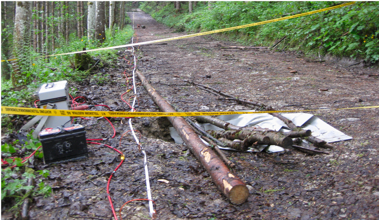
Fig. 1. Picture of the provisionally covered entrance of Forststraßeneinbruch, also visible the ERT instrument and the cables.
