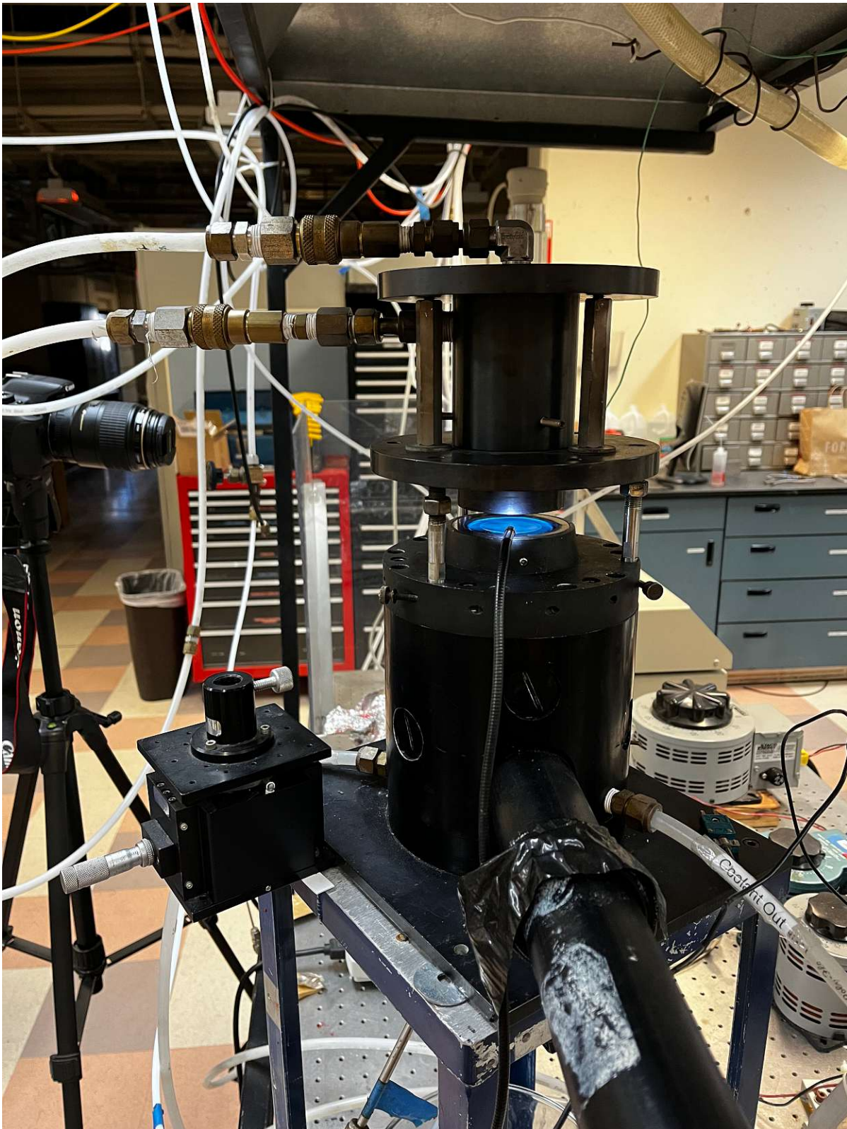
Fig. 3.4: Counterflow burner in extinction configuration at fixed O_2 mass fraction Y_{O_2,2} = 0.195 of 50%Vol.Heptane–50%Vol.Ethanol mixture
