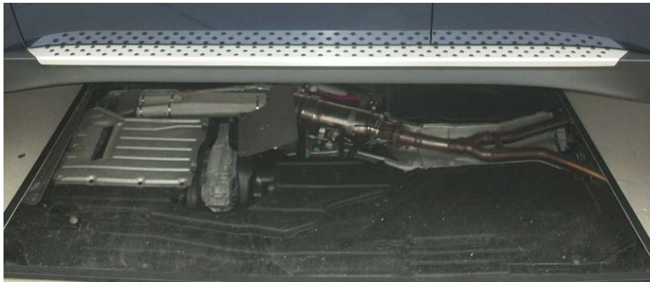
Figure 1.1: A 200 W thermoelectric generator is used in BMW's automobile (The 31st international and 10th European conference on thermoelectrics, July 9-12, 2012, Aalborg, Denmark).
