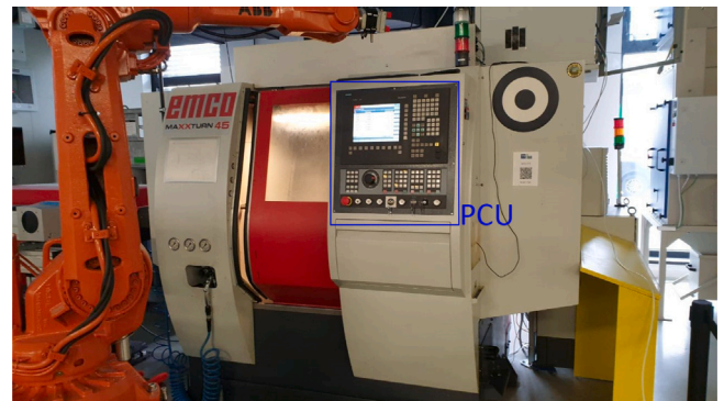
Fig. 2. The turning machine of the pilot factory in Vienna, Austria (in operation). In the blue box, there is the PCU. The NCU is mounted inside, on the rear.
