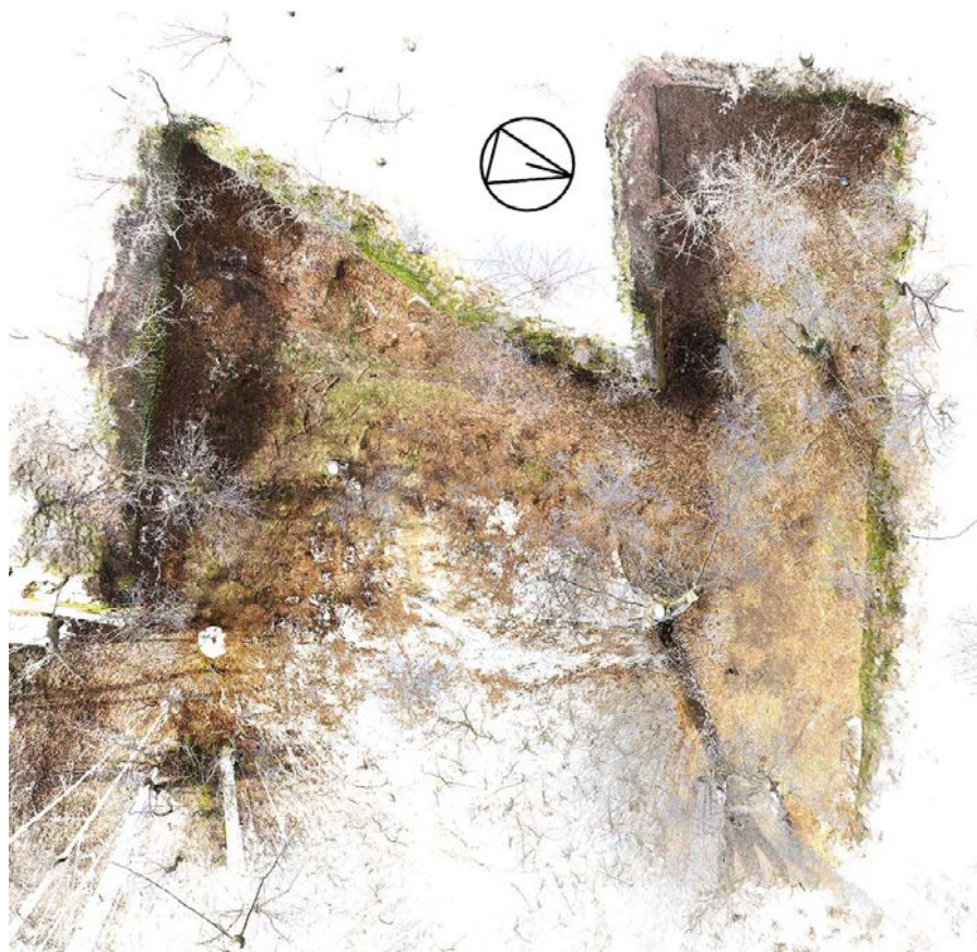
Figure 4. Point cloud overview of the 1225 m 2 area of the abandoned quarry; the point could serve as a basis for a ground floor plan and as a general 3D documentation.
