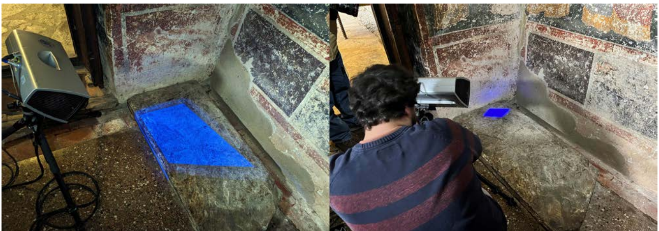
Figure 6. Scanning the gravestone of St. Kliment in Ohrid using the Comet L3D 5M with two different resolutions and, therefore, different areas to capture, left: 260 mm x 215 mm at 0.1 mm point spacing, right: 74 mm x 62 mm at 0.03 mm point spacing.
