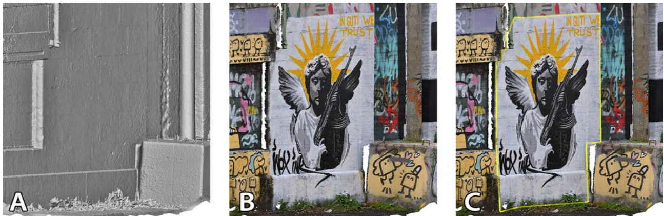
Figure 22. AUTOGRAF can compute a 3D surface mesh (A) with texture (B) from the series of overlapping photos acquired per graffito. On this textured mesh, the GRAPHIS image polygon can be projected (C) to yield a 3D closed polyline whose vertices have real-world 3D coordinates.
