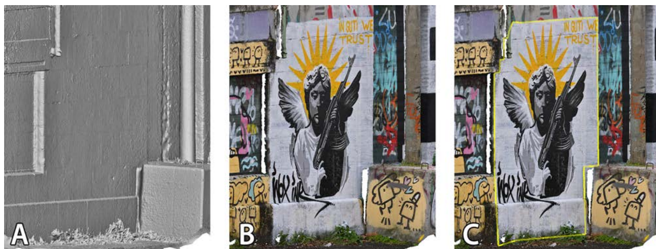
Figure 7. AUTOGRAF can compute a 3D surface mesh (A) with texture (B) from the series of overlapping photos acquired per graffiti. On this textured mesh, the image polygon can be projected (C) to yield a 3D closed polyline of which the vertices have real-world 3D coordinates.
