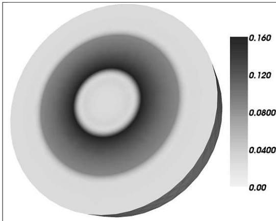
Figure 6.10: Magnetic field distribution at 30 GHz.
