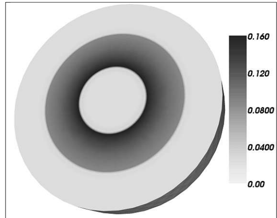
Figure 6.11: Magnetic field distribution at 300 GHz.
