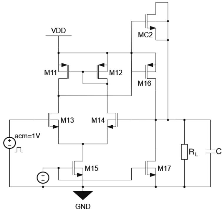
**Figure 8.4:** Schematic used for the simulation of the isolated buffer amplifier. Voltage biasing is provided by voltage sources at the gates of M13, M15 and M17. The voltage source at the gate of M13 has an AC magnitude (acm) of 1 V for AC analysis, and it also generates voltage pulses for transient analysis.
