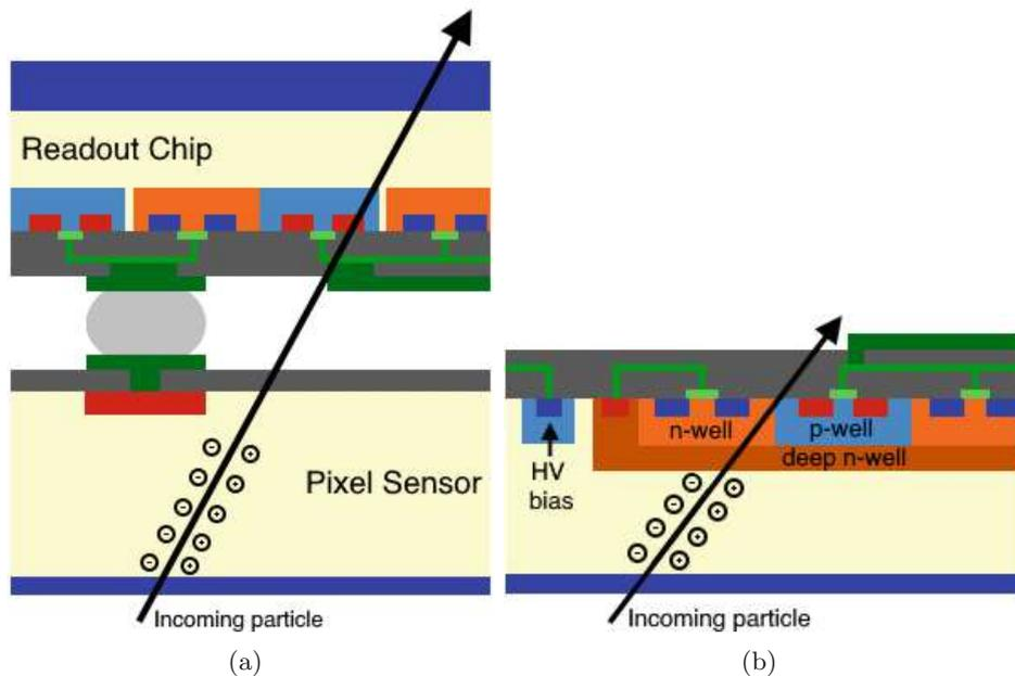
**Figure 2.7:** Schematic cross section of a (a) hybrid pixel detector consisting of separate chips for the sensor and readout electronics and (b) monolithic active pixel sensor integrating the sensor and readout on the same chip.
