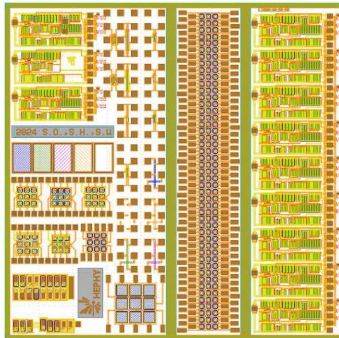
**Figure 12.1:** Chip layout design for the MPW production run via Europractice and Fraunhofer IISB, including the presented CSA circuit layout. Several copies of the CSA layout are implemented along the right edge of the die as well as in the upper-left corner.
