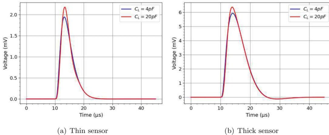
**Figure 9.4:** Output signal of the full CSA for four combinations of sensor configurations and load capacitances  $C_L$  – (a) thin sensor configuration: signal charge  $Q_{in} = 662 e^-$  and input capacitance  $C_{in} = 1\text{ pF}$ ; (b) thick sensor configuration: signal charge  $Q_{in} = 2755 e^-$  and input capacitance  $C_{in} = 4.5\text{ pF}$ .
