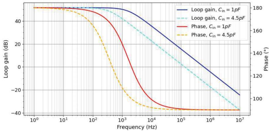
**Figure 9.1:** Loop gain and phase as a function of the frequency of the full CSA for an input capacitance  $C_{in}$  of 1 pF and 4.5 pF.
