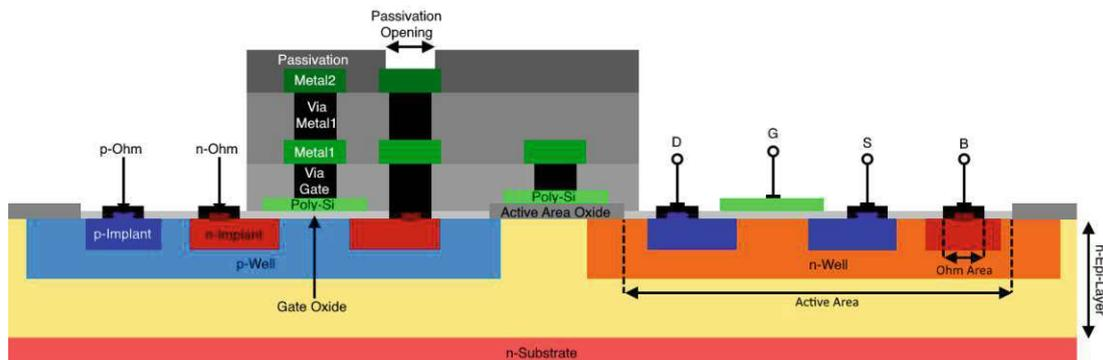
**Figure 6.1:** Visualisation of the used technology, including the available implants and layers and a possible implementation of NMOS and PMOS transistors.
