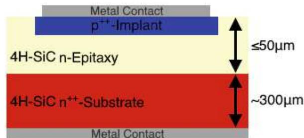
**Figure 2.5:** Cross-section of a p-in-n SiC particle sensor diode consisting of a n-doped epitaxial layer as the depleted sensor volume grown on a thick and highly doped n-type bulk substrate.
