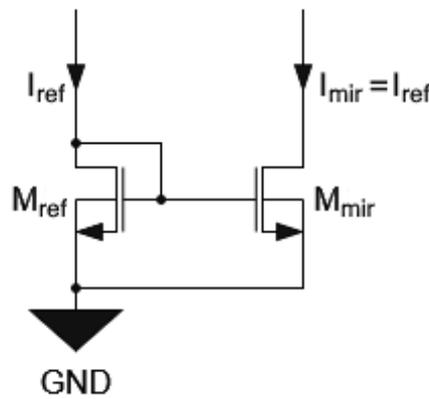
**Figure 5.14:** Basic schematic of a current mirror.
