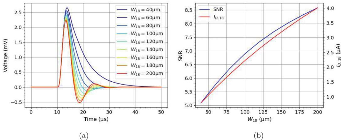
**Figure 8.11:** (a) Simulated output signals and (b) SNR as well as drain current  $I_{D,18}$  of M18 over a sweep of the width  $W_{18}$  of M18 –  $W_{19} = 470 \mu\text{m}$ ,  $W_{C1} = 13 \mu\text{m}$  were used as the widths for M19 and MC1.
