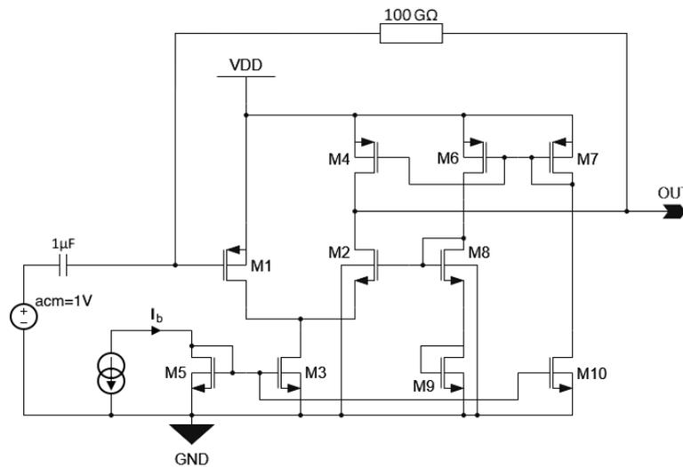
**Figure 8.2:** Schematic used for the simulation of the isolated core amplifier with biasing network. Biasing is provided by a biasing network supplied by externally provided biasing current  $I_b$ , which is represented as a DC current source in the schematic.
