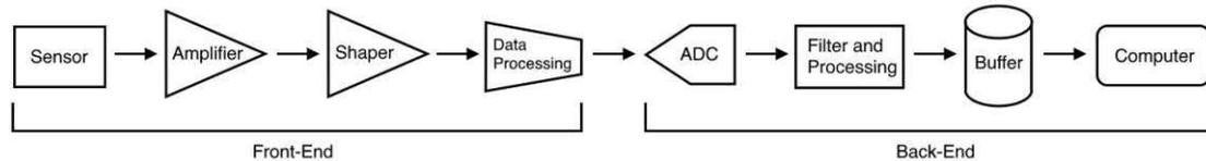
**Figure 2.6:** Schematic of a typical readout chain for particle detectors.
