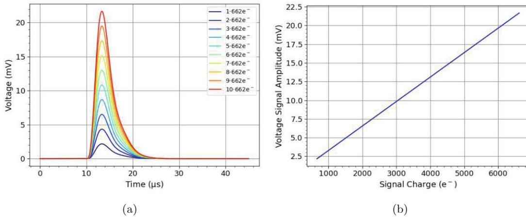
**Figure 9.5:** (a) 10 output signals and (b) corresponding signal amplitudes for linearly increasing signal charge – an input capacitance of  $C_{in} = 1$  pF and load capacitance of  $C_L = 20$  pF were used.
