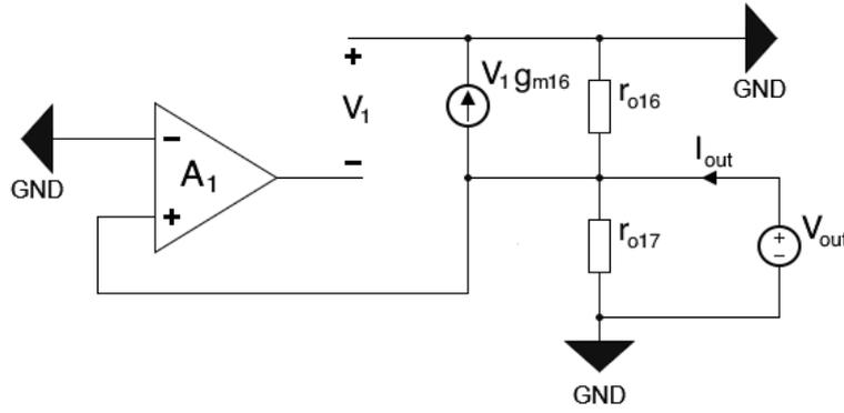
**Figure 5.13:** Small signal circuit for the calculation of the output resistance of the buffer amplifier.
