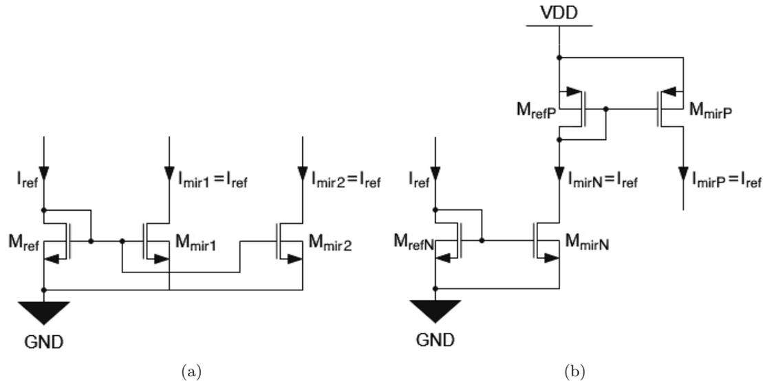
**Figure 5.15:** Schematic of (a) a current mirror with two mirroring devices and (b) an NMOS current mirror providing a reference current for a PMOS current mirror.
