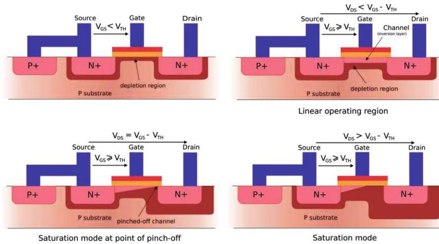
**Figure 3.2:** Visualization of the operation regions of a MOSFET: cut-off (top-left), linear region (top-right), saturation (bottom left), saturation after pinch-off (bottom right). Image adapted from [24].
