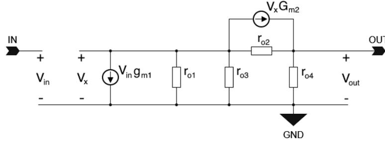
**Figure 5.6:** Small-signal model circuit of the core amplifier.
