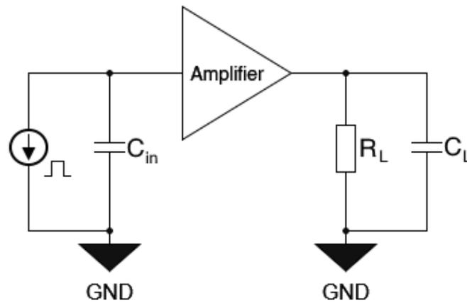
**Figure 5.3:** Schematic of the equivalent circuit of an amplifier with a particle sensor with sensor capacitance  $C_{in}$  at the input and load impedance  $R_L$ ,  $C_L$  at the output.
