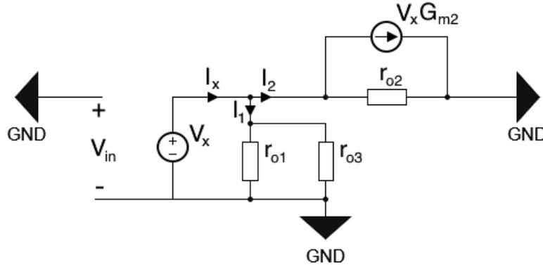
**Figure 5.11:** Grounding the input and output node and applying a voltage  $V_x$  to the folded node in the small-signal model to determine the resistance looking into the folded node of the core amplifier.
