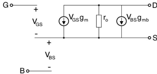
**Figure 3.4:** Small-signal equivalent circuit of a MOSFET.
