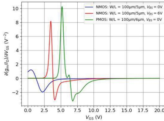
**Figure 6.4:** Derivative of the transconductance-efficiency  $\frac{\partial(g_m/I_D)}{\partial V_{GS}}$  as a function of the gate-source voltage  $V_{GS}$  of an NMOS transistor, a PMOS transistor and an NMOS transistor with bulk-source voltage  $V_{BS} = 6$  V - the widths of all the transistors is  $100 \mu\text{m}$ , while the length is  $5 \mu\text{m}$  for the NMOS transistors and  $6 \mu\text{m}$  for the PMOS transistor, respectively.
