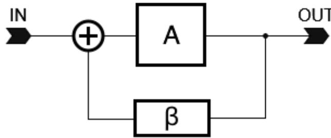
**Figure 4.4:** Generalized schematic of an amplifier  $A$  with a feedback network with the feedback factor  $\beta$ .
