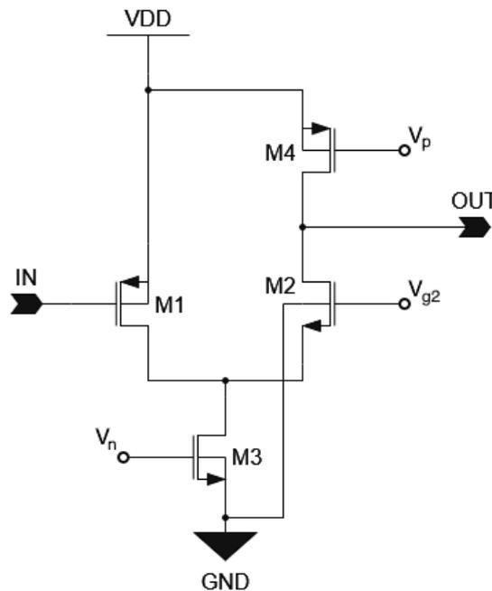
**Figure 5.4:** Schematic of the core amplifier.
