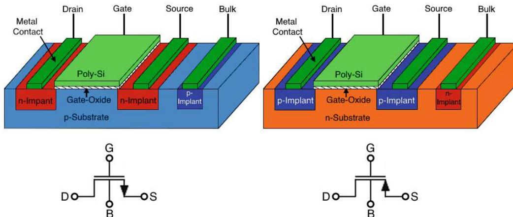
**Figure 3.1:** Cross section and circuit symbol of an n-channel MOSFET (left) and p-channel MOSFET (right)
