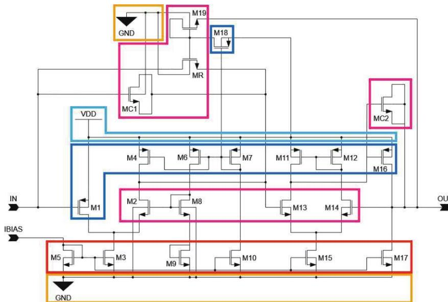
**Figure 10.5:** Grouping of MOSFET structures and circuit nodes for the organization of placement regions in the layout floorplan – Light blue: VDD rail, orange: GND rail, dark blue: PMOS transistors with source and bulk connected to the VDD rail, red: NMOS transistors with source and bulk connected to the GND rail, magenta: MOSFETs with gate, source and drain connected to nodes other than VDD and GND.
