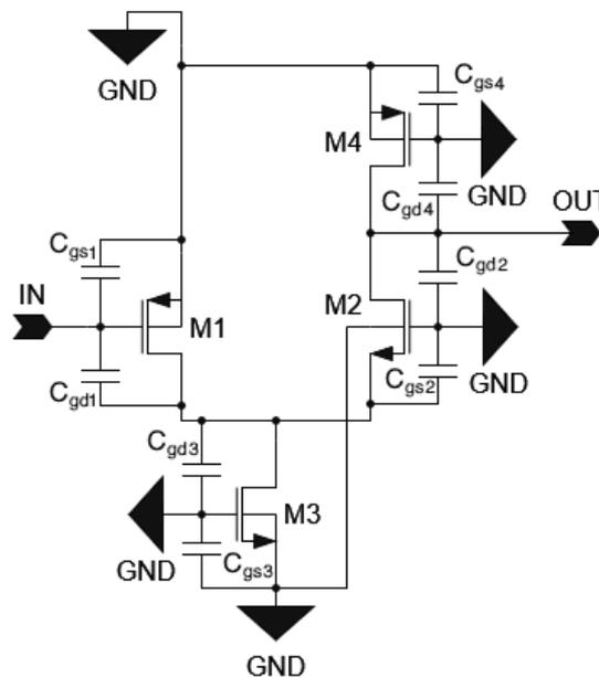
**Figure 5.9:** Setting constant potentials to ground and including parasitic capacitances for determining the high-frequency small-signal model of the core amplifier.
