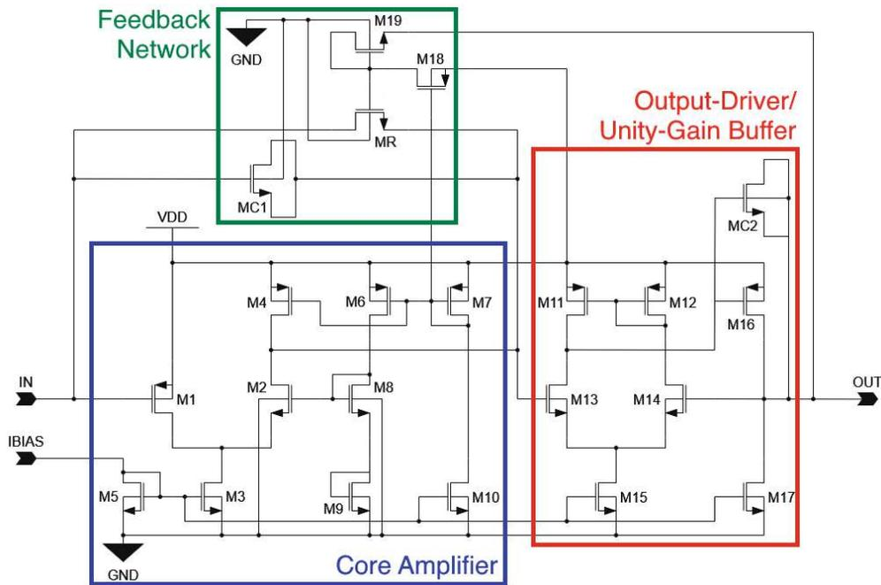
**Figure 5.2:** Full schematic of the CSA.
