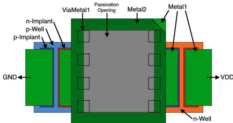
**Figure 5.18:** Layout of a pad with ESD diodes that can be connected to VDD and GND.
