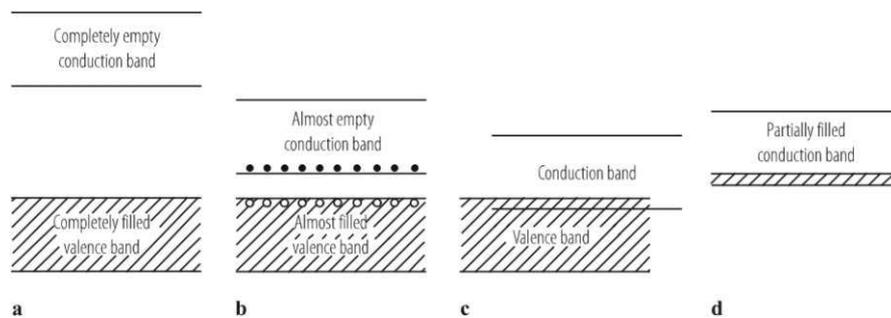
**Figure 2.1:** Visualization of the energy band structure of (a) insulators, (b) semiconductors, and (c), (d) conductors/metals. Image adapted from [15].
