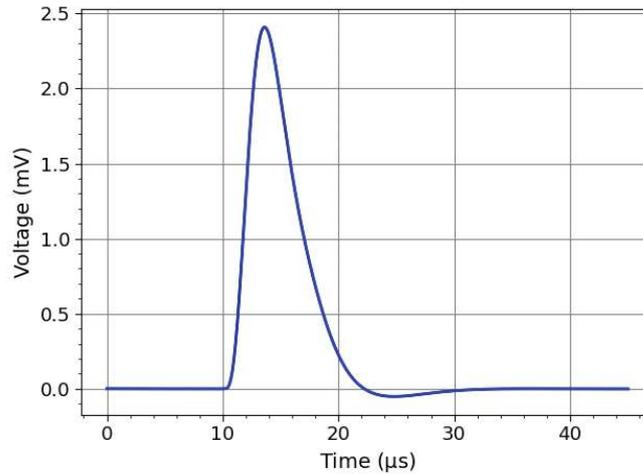
**Figure 8.14:** Simulated output signal of the closed-loop CSA circuit for a signal charge of  $Q_{in} = 662 e^-$ , input capacitance of  $C_{in} = 1 \text{ pF}$  and load capacitance of  $C_L = 20 \text{ pF}$ .
