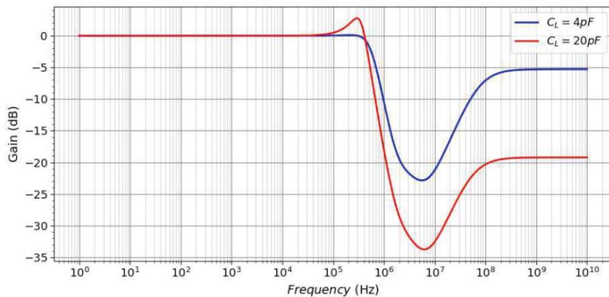
**Figure 8.5:** Gain as a function of frequency for the isolated unity-gain buffer stage.
