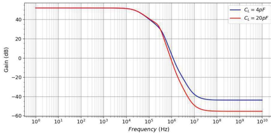
**Figure 8.8:** Gain as a function of frequency for the combination of the core amplifier and buffer amplifier.
