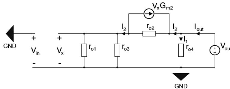
**Figure 5.7:** Grounding the input node and applying a voltage  $V_{out}$  to the output node in the small-signal model, to determine the output resistance of the core amplifier.
