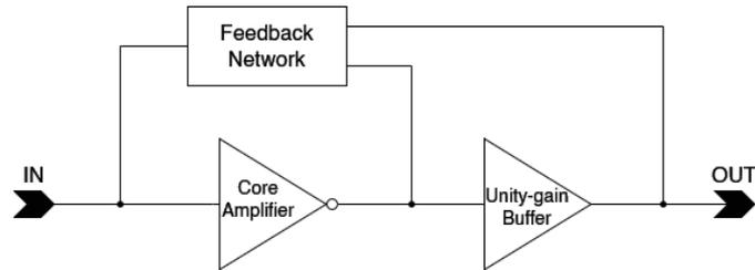
**Figure 5.1:** Simplified overview of the CSA, consisting of the core amplifier, the output driver stage (unity-gain buffer) and the feedback network.
