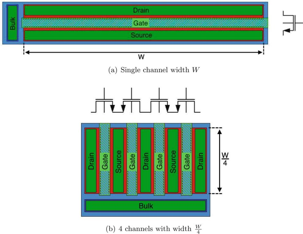
**Figure 10.2:** Layout of an NMOS with (a) a single channel of a width of  $W$  and (b) a finger structure i.e. a width of  $W$  divided onto 4 channels of width  $\frac{W}{4}$  as well as the equivalent circuit schematics – blue: p-Well, dark blue: p-Implant, red: n-Implant, lime (hatched and solid): Poly-Si, green: Metal1.
