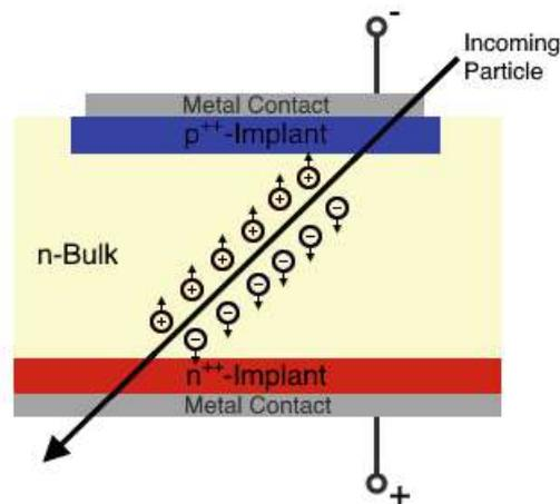
**Figure 2.3:** Structure of a simple semiconductor sensor pixel and the deposition of electron-hole pairs by an incoming high energetic particle.
