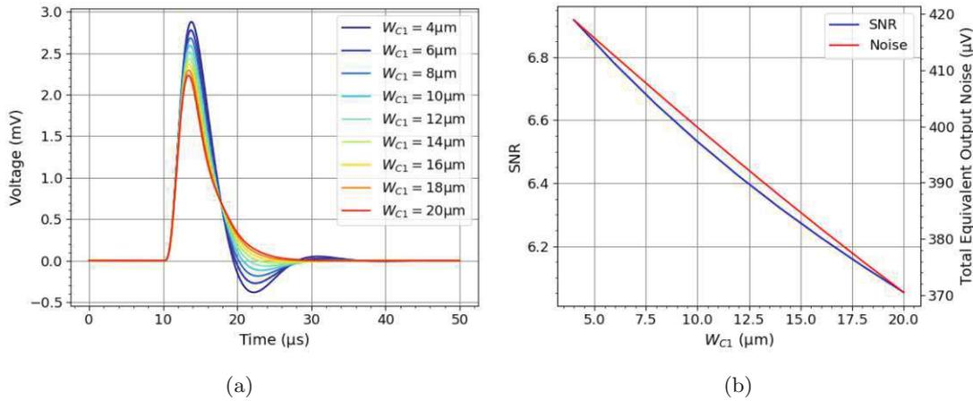
**Figure 8.13:** (a) Simulated output signals and (b) SNR as well as total equivalent output noise of the CSA over a sweep of the width  $W_{C1}$  of MC1 –  $W_{18} = 80 \mu\text{m}$ ,  $W_{19} = 470 \mu\text{m}$  were used as the widths for M18 and M19.
