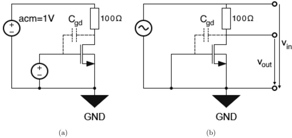
**Figure 6.5:** Schematic used for the extraction of the parasitic gate-drain capacitance  $C_{gd}$  of an NMOS by inserting a small resistance of 10  $\Omega$  to the drain of the MOSFET forming a low-pass filter with the parasitic capacitances and applying an AC signal - (a) simulation schematic with a voltage source with an AC magnitude (acm) of 1 V (b) equivalent circuit in terms of AC signal i.e. static potentials are shorted to GND.
