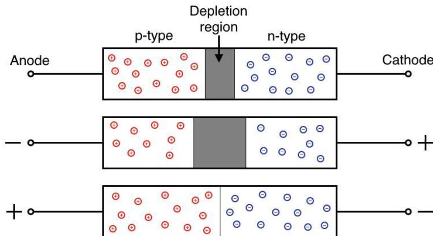
**Figure 2.2:** Manipulation of the depletion region of a diode without external bias (top), reverse bias (center) and forward bias (bottom).
