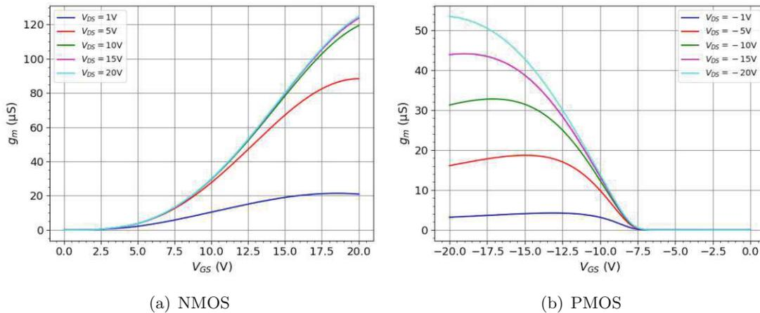
**Figure 6.3:** Simulated transconductance for different drain-source voltages  $V_{DS}$  of SiC NMOS and PMOS with a channel width of  $100\ \mu\text{m}$  and length of  $6\ \mu\text{m}$  at a temperature of  $25^\circ\text{C}$  and bulk-source voltage  $V_{bs} = 0\ \text{V}$  [36].
