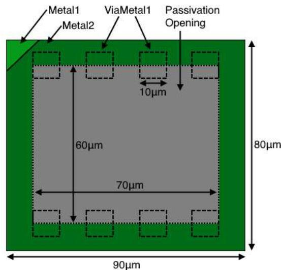
Figure 5.17: Layout of a pad used to bias the CSA and bring signals to and from the CSA.
