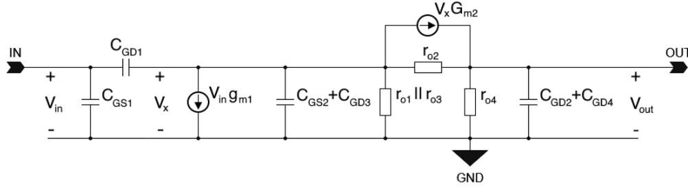
**Figure 5.10:** High frequency small-signal model of the core amplifier.
