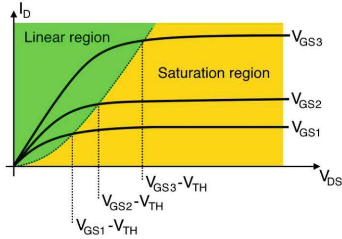
**Figure 3.3:** Visualization of the output characteristics of a MOSFET, i.e. the drain current  $I_D$  as a function of its drain-source voltage  $V_{DS}$  for different gate-source voltages  $V_{GS}$ .  $I_D$  begins to saturate as  $V_{DS}$  approaches  $V_{GS} - V_{TH}$ .
