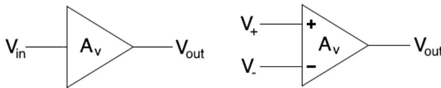
**Figure 4.1:** Single-ended amplifier (left) and differential amplifier with single-ended output (right) with a voltage gain of  $A_v$ .
