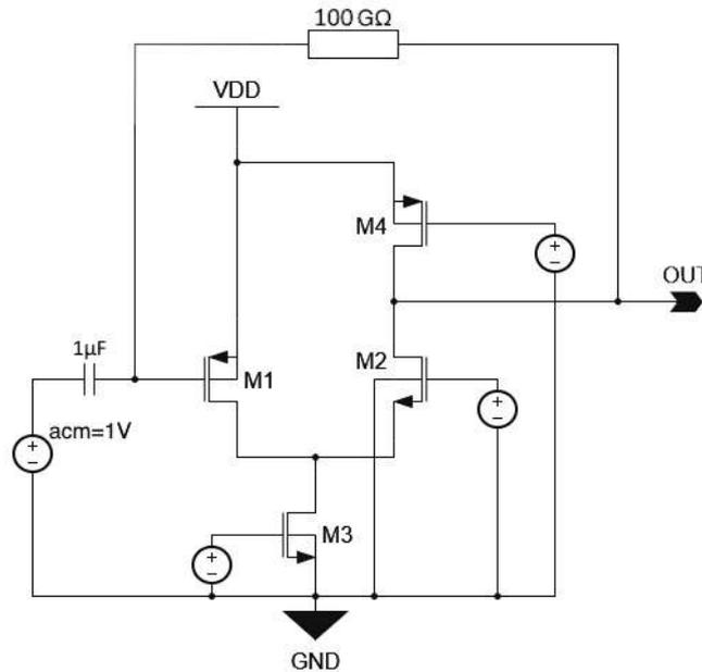
**Figure 8.1:** Schematic used for the simulation of the isolated core amplifier. Biasing is provided by voltage sources at the gates of M2, M3 and M4. M1 is biased by a high ohmic connection of its gate to the output node. For AC analysis, a voltage source with AC magnitude (*acm*) of 1 V is AC coupled to the input of the amplifier.
