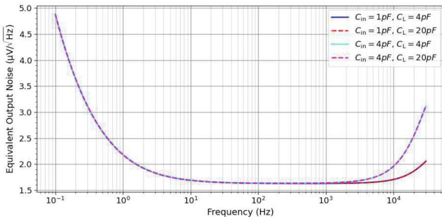
**Figure 9.3:** Equivalent output noise voltage as a function of the frequency of the full CSA for four combinations of input capacitance  $C_{in}$  and load capacitance  $C_L$ .
