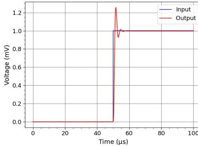
**Figure 8.6:** Step response of the unity-gain buffer stage with a load capacitance of  $C_L = 20$  pF - step input signal of 1 mV in blue and response output signal in red.
