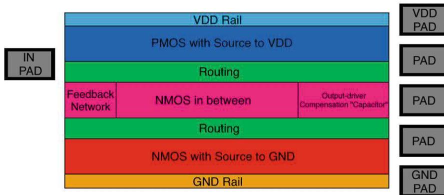
**Figure 10.6:** Rough layout floorplan of the CSA based on the circuit schematic.
