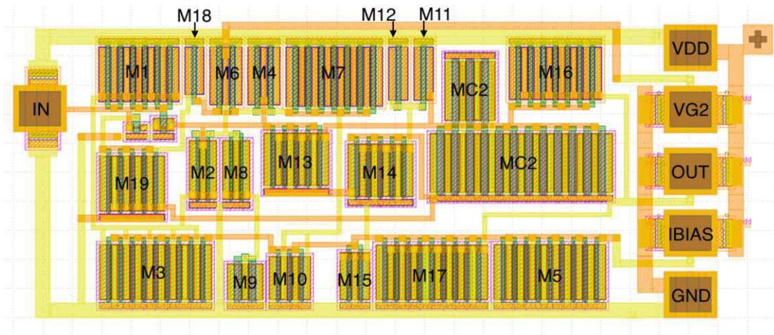
**Figure 10.7:** Finished layout of the CSA including labelling of all MOSFETs and Pads – yellow wires are on the Metal1 layers and the orange wires are on the Metal2 layer.
