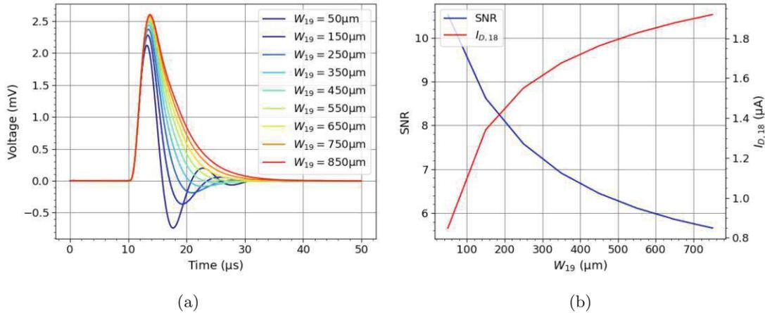
**Figure 8.12:** (a) Simulated output signals and (b) SNR as well as drain current  $I_{D,18}$  of M18 over a sweep of the width  $W_{19}$  of M19 –  $W_{18} = 80 \mu\text{m}$ ,  $W_{C1} = 13 \mu\text{m}$  were used as the widths for M18 and MC1.
