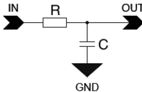
**Figure 4.2:** Circuit of a low-pass RC-circuit with a resistor  $R$  and a capacitance  $C$ .
