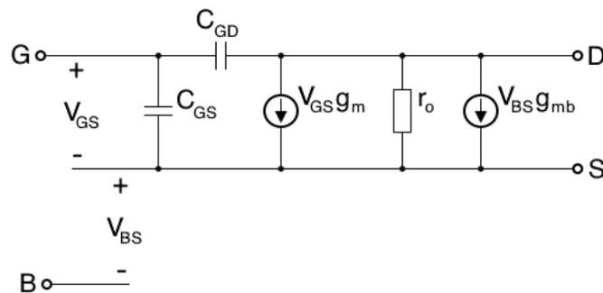
**Figure 3.5:** Small-signal equivalent circuit of a MOSFET at high signal frequencies.
