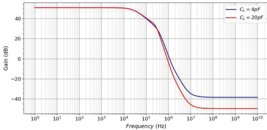
**Figure 9.2:** Gain as a function of the frequency of the full CSA for a load capacitance  $C_L$  of 4 pF and 20 pF.
