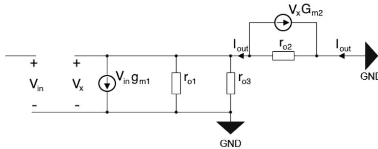
**Figure 5.8:** Grounding the output node with an output current  $I_{out}$  flowing into the circuit of the small-signal for the determination of the equivalent transconductance of the core amplifier.
