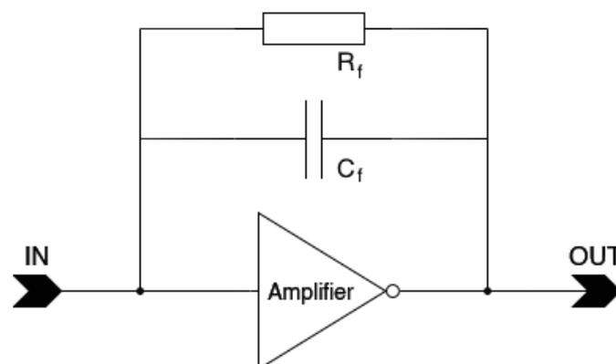
Figure 4.5: Schematic of a charge sensitive amplifier.
