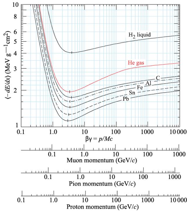
**Figure 2.4:** Mean energy loss of a muon, pion and proton in different materials as a function of the particle momentum modeled by the Bethe-Bloch equation. Image Adapted from [18].
