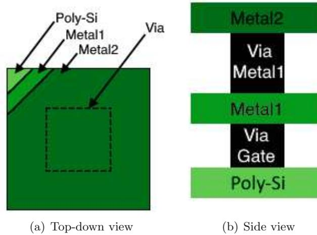
**Figure 10.1:** Via stack consisting of a  $12 \cdot 12 \mu\text{m}^2$  Poly-Si layer on the bottom, a ViaGate1 with dimensions of  $4 \cdot 4 \mu\text{m}^2$  connecting to a  $12 \cdot 12 \mu\text{m}^2$  Metal1 layer and a  $4 \cdot 4 \mu\text{m}^2$  ViaMetal1 connecting  $12 \cdot 12 \mu\text{m}^2$  Metal2 layer - the dashed lines in (a) enclose the cross-sectional area of both vias stacked over each other.
