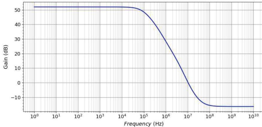
**Figure 8.3:** Gain as a function of frequency for the core amplifier.
