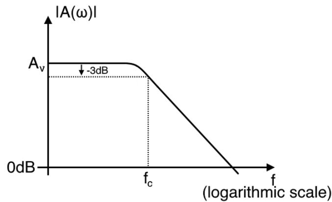
**Figure 4.3:** Visualization of the gain magnitude  $|A(\omega)|$  as a function of frequency  $f$  with a logarithmic frequency scale. For  $f \ll f_c$ , the gain equals the DC voltage gain  $A_v$ .
