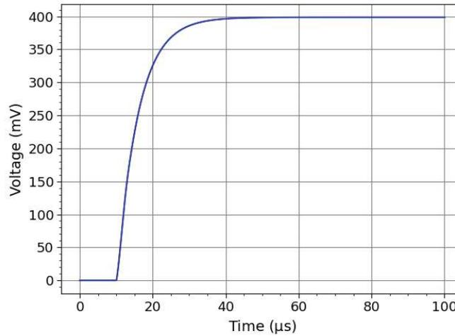
**Figure 8.9:** Voltage signal response of the combined core amplifier and unity-gain buffer to a step input signal of 1 mV.
