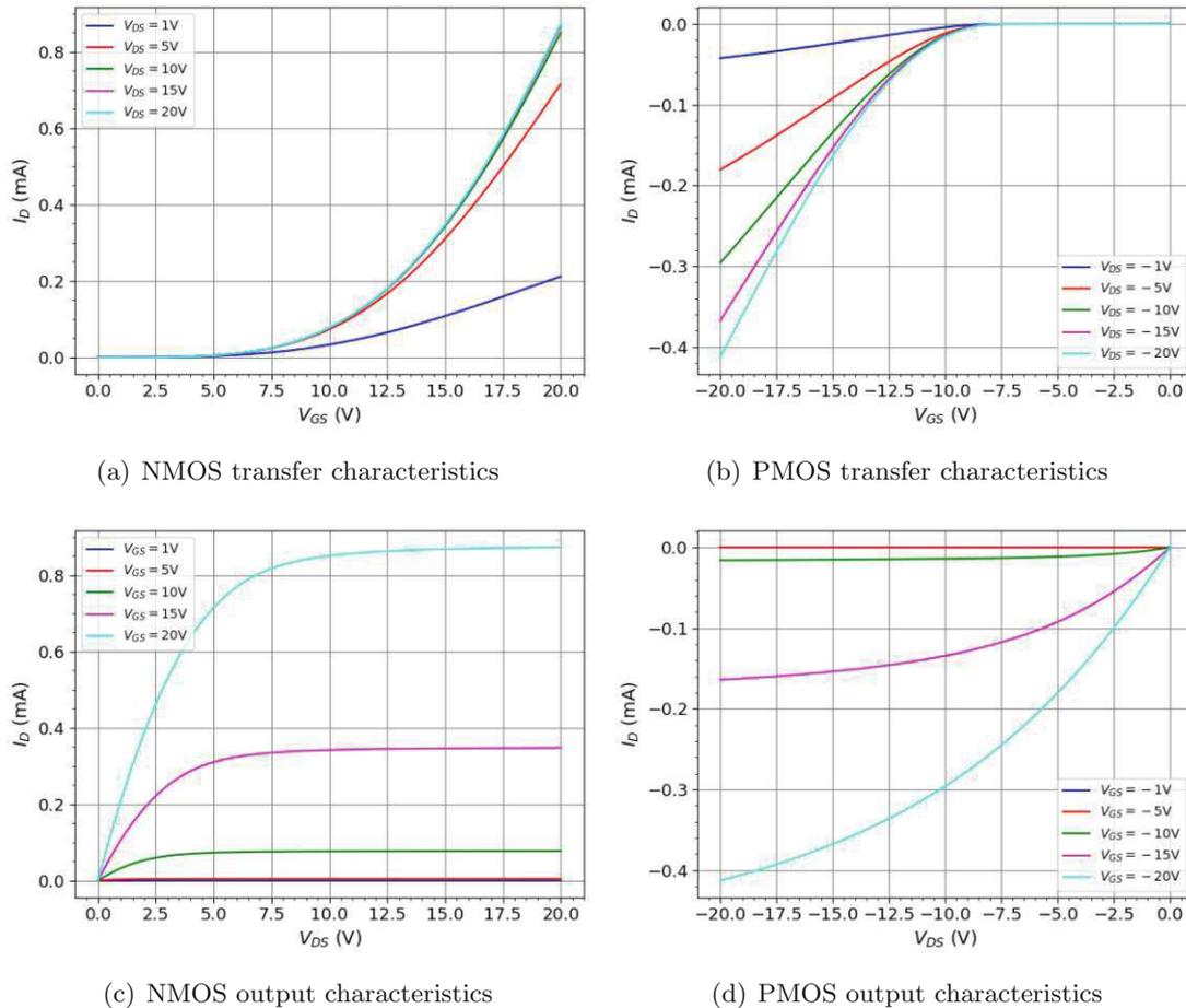
**Figure 6.2:** Simulated (a),(b) transfer characteristics and (c),(d) output characteristics of SiC NMOS and PMOS transistors with a channel width of  $100\ \mu\text{m}$  and length of  $6\ \mu\text{m}$  at a temperature of  $25\ ^\circ\text{C}$  and bulk-source voltage  $V_{bs} = 0\ \text{V}$  [36].
