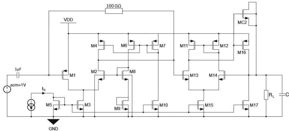
**Figure 8.7:** Schematic used for the simulation of the buffer amplifier with biasing network i.e. a combined core and buffer amplifier without the feedback network. Biasing is provided by a biasing network supplied by externally provided biasing current  $I_B$ , which is represented as a DC current source in the schematic. For AC analysis, a voltage source with AC magnitude (acm) of 1 V is AC coupled to the input of the core amplifier.
