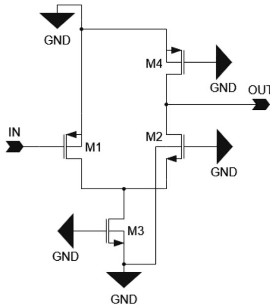
**Figure 5.5:** Setting constant potentials to ground for the determination of the small-signal model of the core amplifier.
