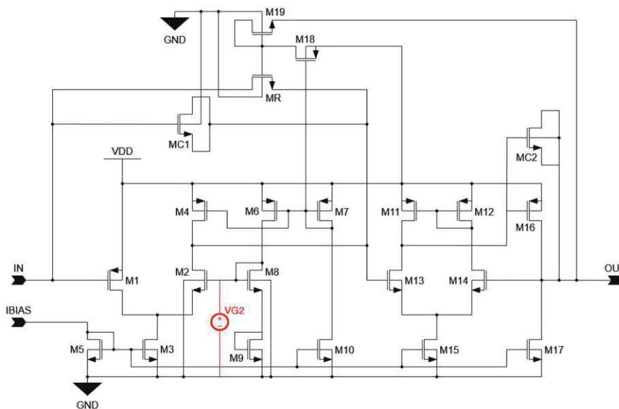
**Figure 10.4:** Equivalent circuit schematic of the CSA if an additional external voltage supply VG2 (red) is introduced to the gate of M2 via an additional bonding pad on the layout.
