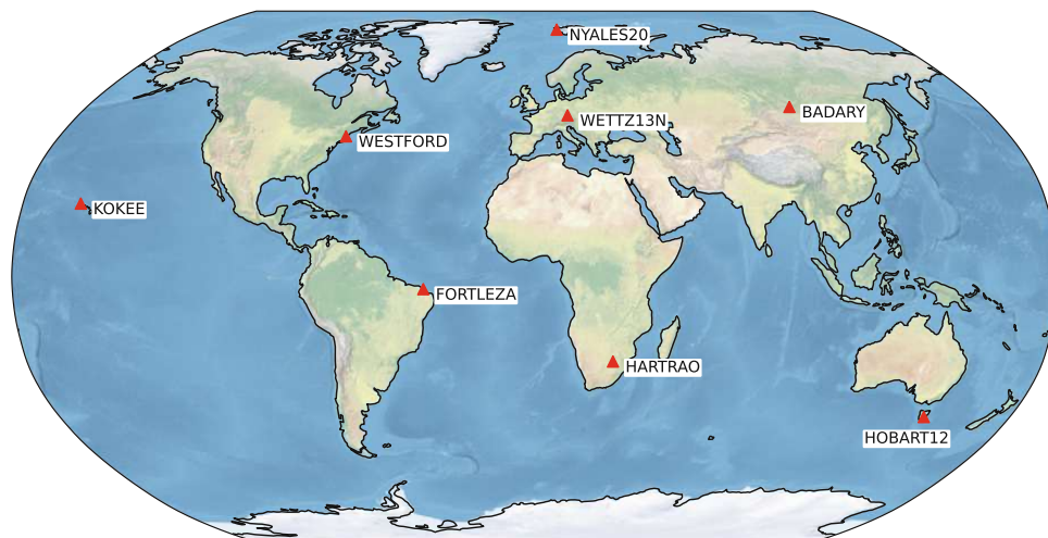
Figure 4.1: Positions of the VLBI stations for the visibility study. The selected VLBI stations are regularly part of IVS-R1 or IVS-R4 sessions.
