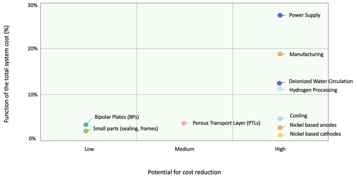
Figure 3.1 - system components for a 1MW alkaline electrolyzer classified based on their contribution to total system costs and potential for cost reduction (derived from IRENA, 2020, p.56)
