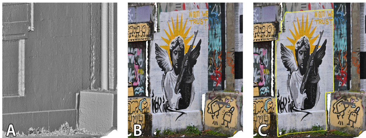
Figure 7. AUTOGRAF can compute a 3D surface mesh (A) with texture (B) from the series of overlapping photos acquired per graffito. On this textured mesh, the image polygon can be projected (C) to yield a 3D closed polyline of which the vertices have real-world 3D coordinates.
