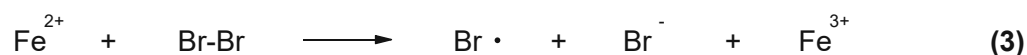
Figure 10: Scheme of Fenton like reaction between Fe(II) and a disulfide (1), a disulfone (2) and a halide (3) leading to the respective anions, radicals and Fe(III).
