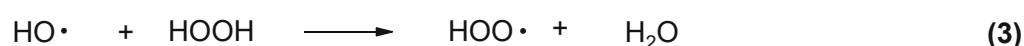
Figure 7: Reaction scheme of the Fenton reaction. (1): reaction of Fe(II) with hydroperoxide, leading to a hydroxyl radical, a hydroxyl anion and oxidized Fe(III). (2): side reaction of the hydroxyl radical with Fe(II) leading to a hydroxyl anion and oxidized Fe(III). (3): side reaction of the hydroxyl radical with hydroperoxide leading to a low reactive peroxy radical and water.
