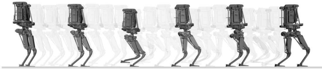
Figure 7.10: Time series of the humanoid robot Kangaroo [7] during a walking to running transition.
