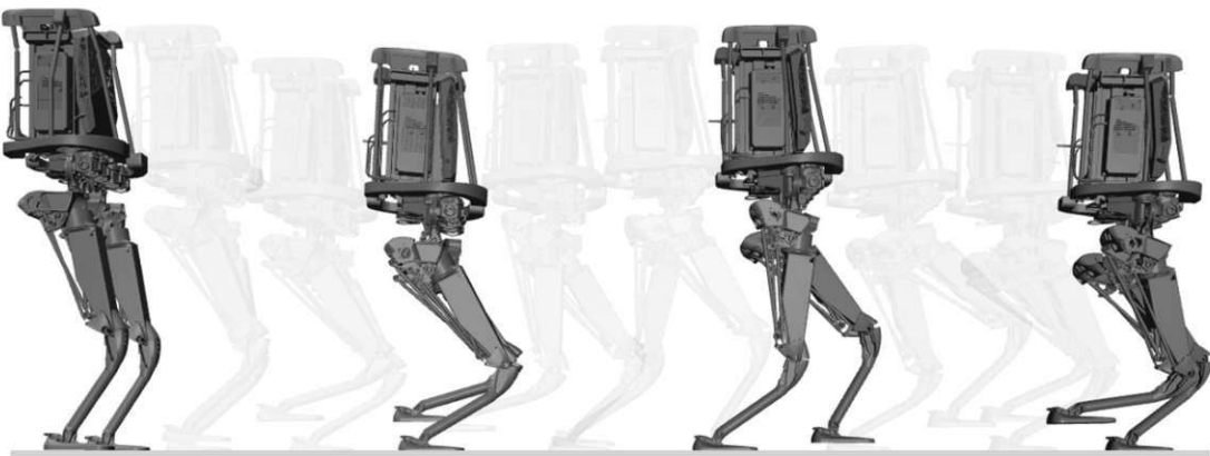
Figure 1.1: Timeseries of humanoid robot Kangaroo [7] while running.
