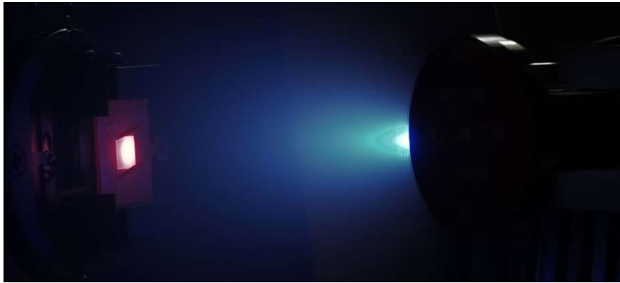
Figure 2.1: Long exposure photograph of multiple plasma plumes (right) ejected from the LSMO target onto an SrTiO 3 sample (left) heated to a temperature of 800°C.
