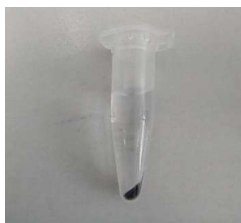
Figure 18: Removal of the reaction components after the Wacker oxidation by centrifugation.
