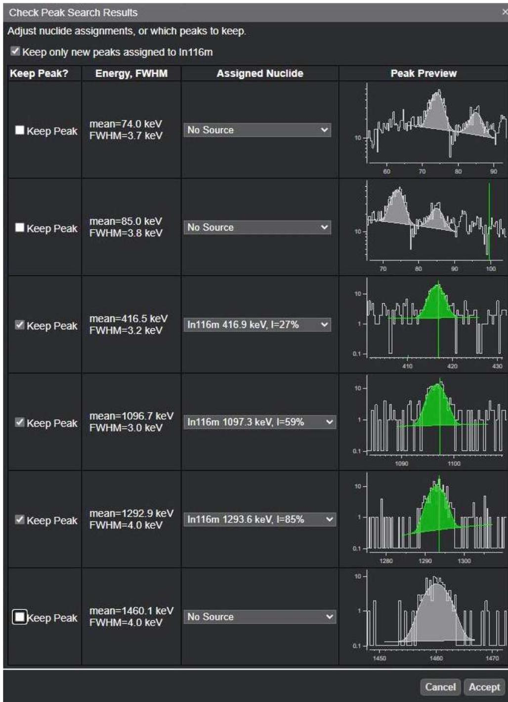
Figure 3.13: Results screen of the peak search algorithm. Peaks at the energies of a reference line are displayed in a chosen colour.
