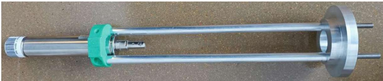
(c) Image of one of the three used VacuTec 70 063  $^3\text{He}$  detectors with mount.
