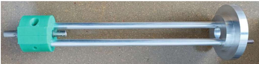
(c) Image of the Canberra 0.5NH1/1KF  $^3\text{He}$  detector with mount.**Figure 3.7:** The Canberra 0.5NH1/1KF  $^3\text{He}$  detector.
