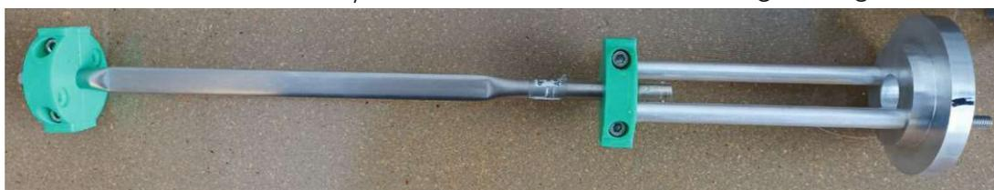
(b) Image of one of the two used Canberra 20NH20/1TP  $^3\text{He}$  detectors with mount.
