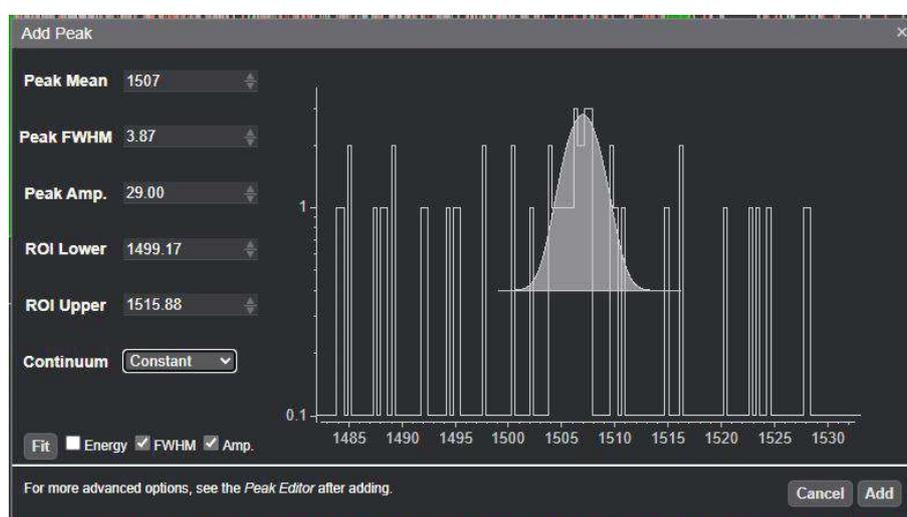
Figure 3.12: Manual addition of a peak at 1507 keV. Due to the low intensity, it is barely discernable from the background.
