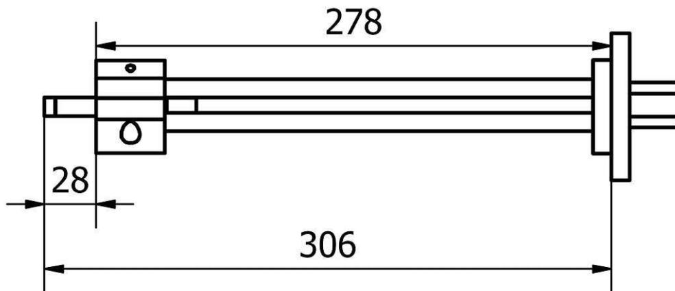
(b) Sketch of the Canberra 0.5NH1/1KF  $^3\text{He}$  detector with mount. Lengths are given in mm.
