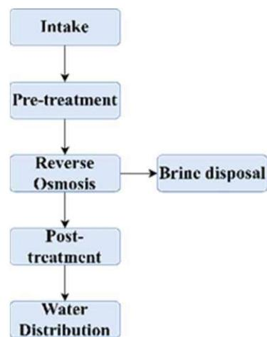
Figure 2. Flow diagram of water desalination.
