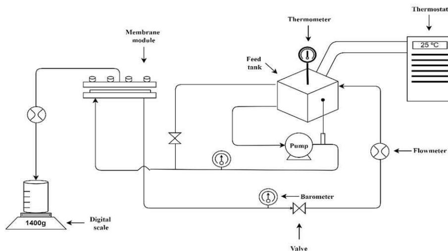
**Figure 1.** Schema of membrane test cell (model OS-MC-01).
