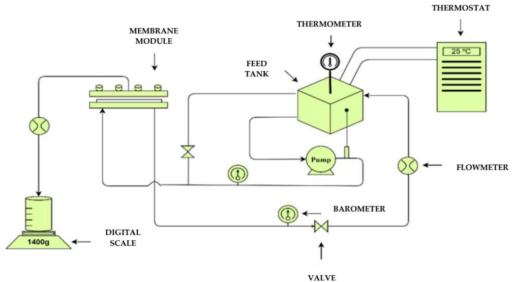
Figure 5. Membrane System Equipment (Model OS-MC-01). Adapted from Cabrera-González et al.
