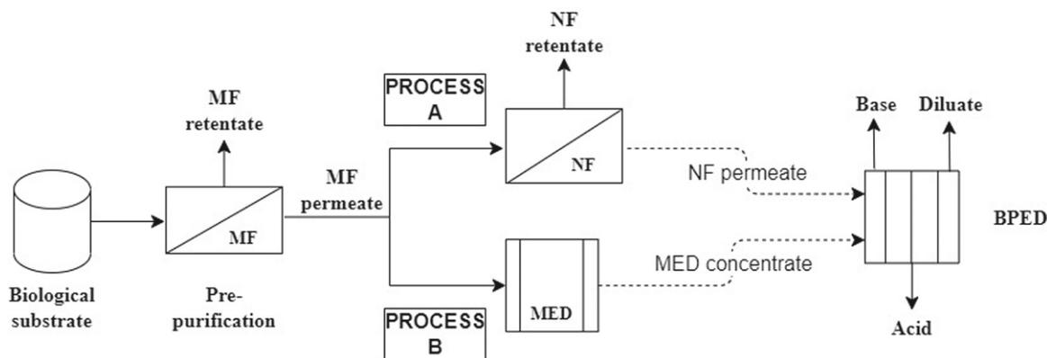
Fig. 1. Experimental set-up for maximum lactic acid recovery and purity.
