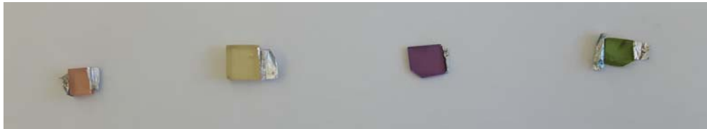
Figure 4.2: Photo of the four langasite a-cut crystals. Silver tape used for mounting is attached to the edges of the samples. From left to right: LGS, HoLGS, NGS, PGS.
