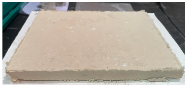
Figure 5. Photo of moulded sample of wood flour core insulation for vacuum insulators
