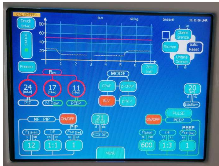
Figure 6: Screen of the ventilator, all fields in light blue can be selected or changed. The orange fields mark what is currently actively selected.
