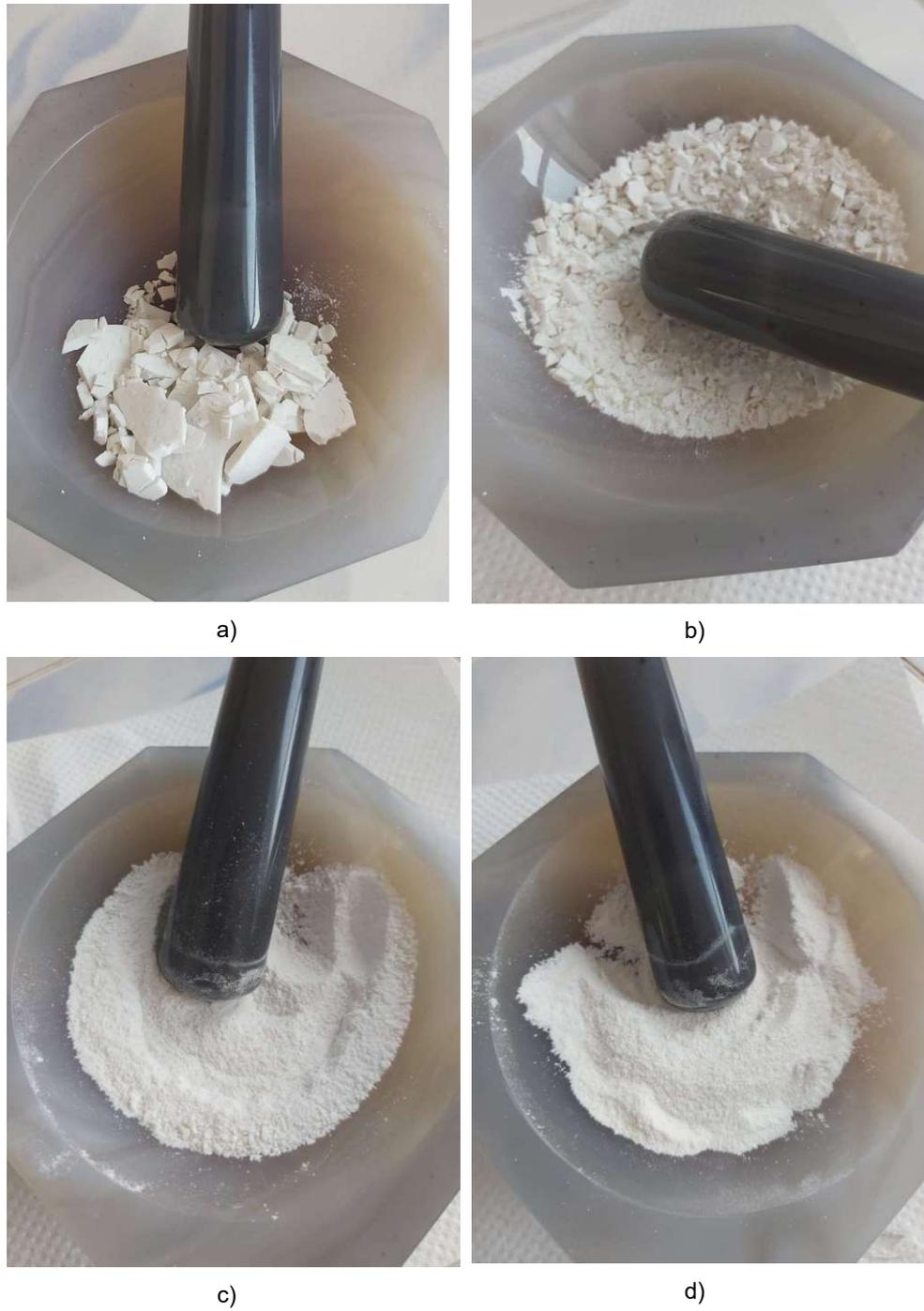
Figure 3.7. Several stages of grinding
