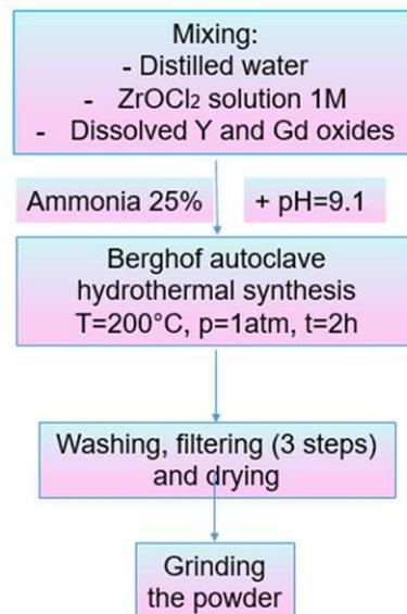
Figure 3.2. Hydrothermal flow for doped zirconia.
