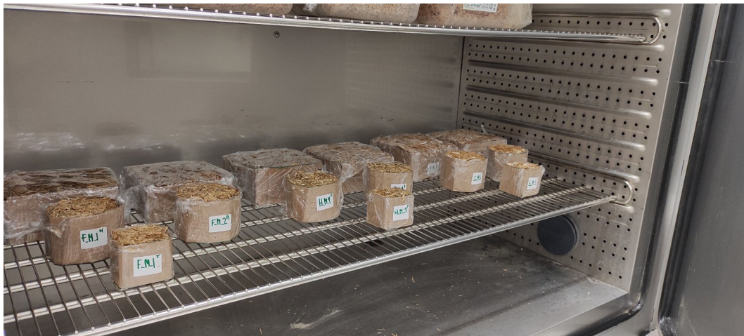
Figure 4. Preparing samples of each type in a climate chamber: wheat, hemp, and flax straw.
