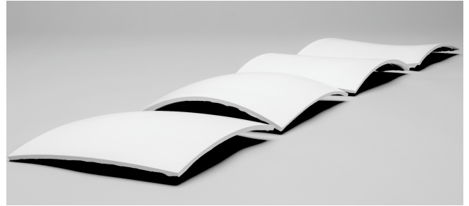
Fig. 13. From left to right, manually fabricated gypsum panels TP1 ( K > 0 ), TP2 ( K \gg 0 ), TP4 ( K < 0 and K > 0 ), and TP3 ( K < 0 ).
