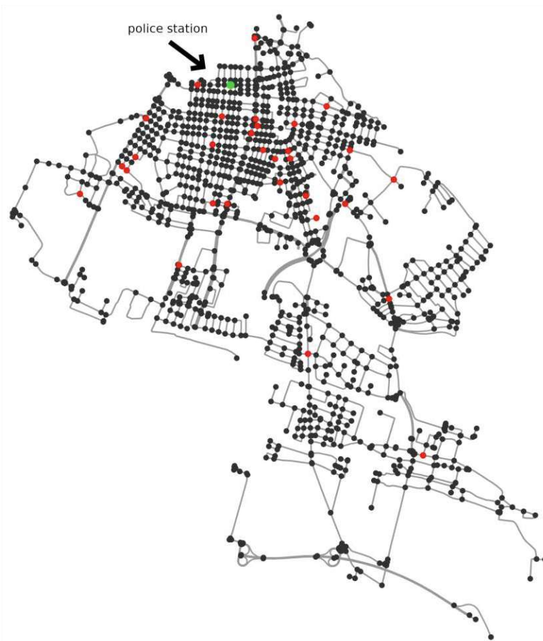
Figure 8: Network graph of the district Favoriten in Vienna, with patrol locations marked in red and the police station marked in green. (Map data © OpenStreetMap)
