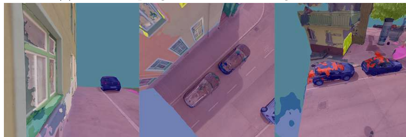
(b) Random sampling. Contains many misclassified areas. Especially sidewalk (pink) is often misclassified as road (purple).
