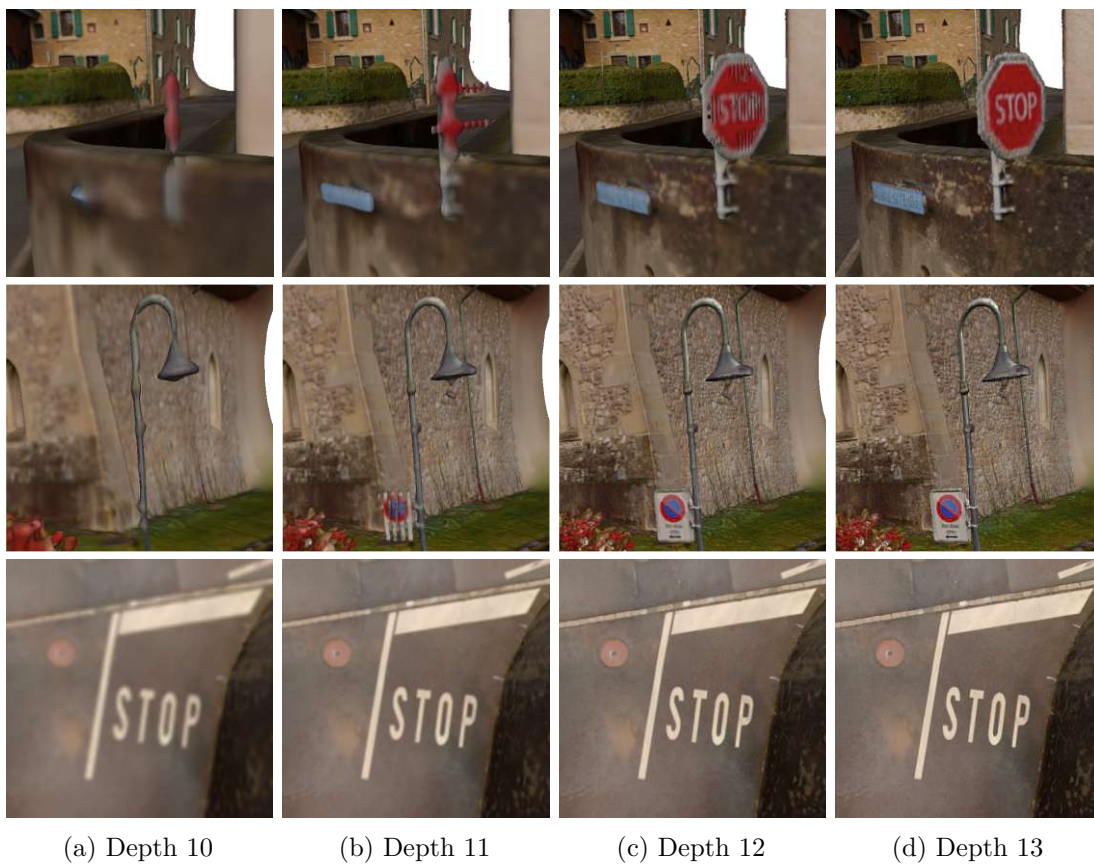
Figure 5.16: Reconstructions from a point cloud at different Poisson depths
