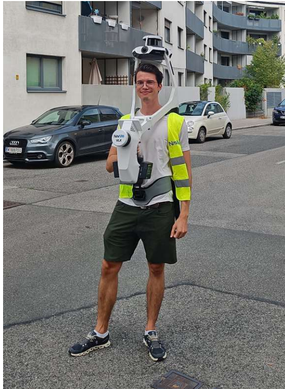
Figure 5.3: The NavVis VLX mobile mapping device
