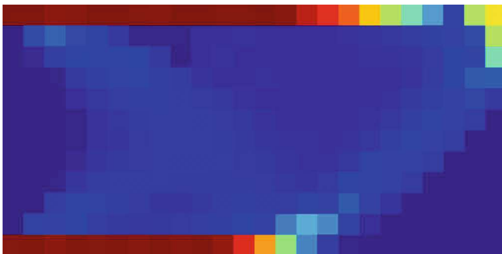
Figure B.2.: Parameter-spline of the optimized geometry with the alternative compliance measure. Here we assigned every tile their parameters individually, which can be interpreted as a zero-th degree spline in the proposed framework.
