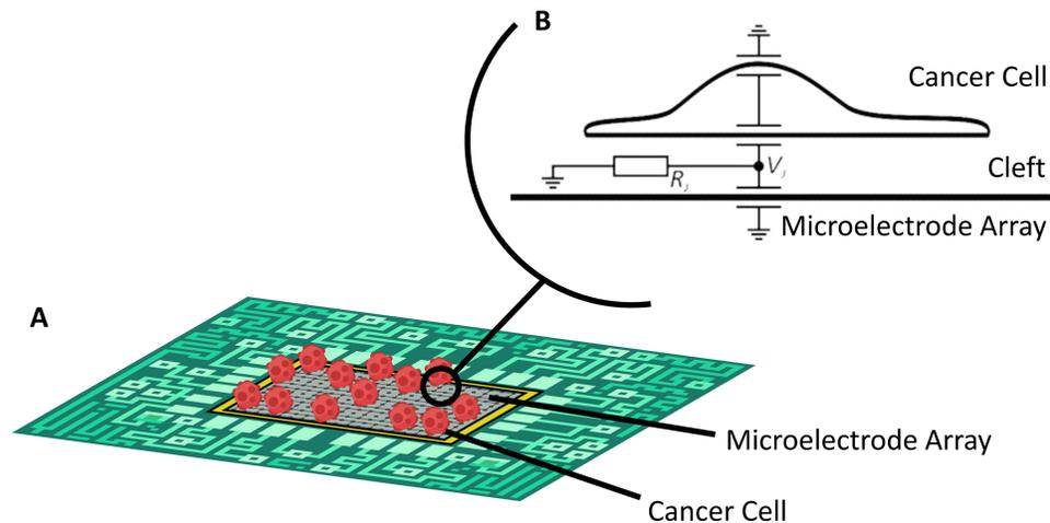
Figure 1: **Cancer cell-CMOS microelectrode array (CMOS MEA) interface.**
