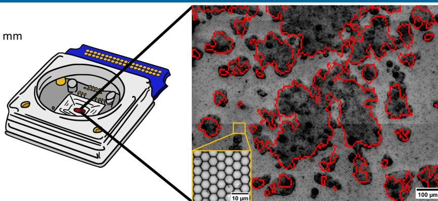
Figure 2: **Non-invasive detection of cell attachment using cell adhesion noise spectroscopy ( $S_V$ , assessed at 300 kHz).** (left) Schematic CMOS microelectrode array (MEA) with high-density recording sites. (right) Overlay of electrically identified HT-29 cells (red contours) with brightfield microscopic image of the CMOS MEA with adherent HT-29 cells (dark grey/black: cell clusters, light grey: sensor sites in the background). Inset: 50x magnification of sensor sites on the MEA. [5]
