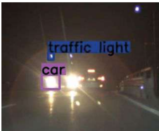
Figure 5.22: Reflections of an approaching car being wrongly classified as traffic lights. The left headlight is misclassified as the complete car.
