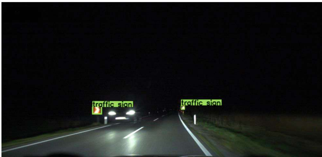
Figure 5.17: Example of object detection from “phase 1”, after merging the 40 different traffic sign classes into one class “Traffic Sign”.
