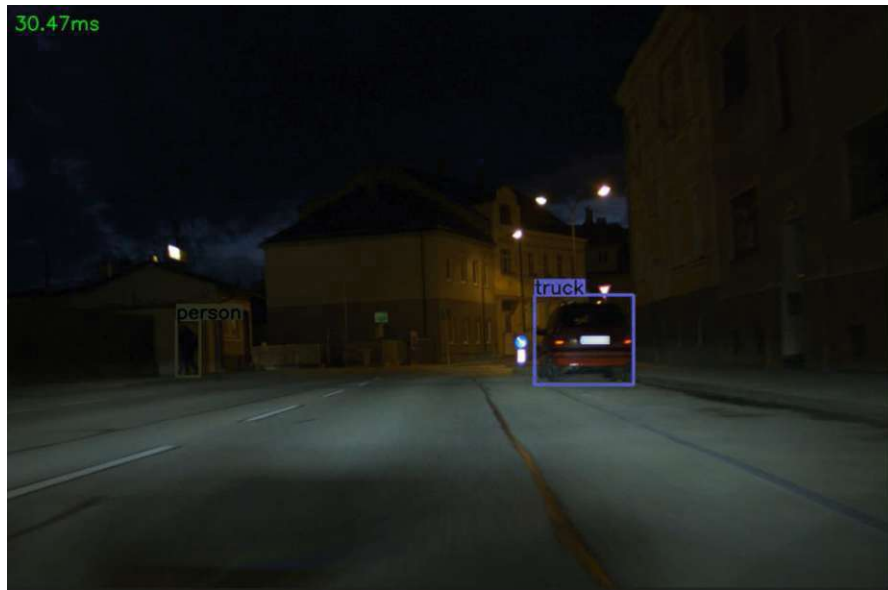
Figure 5.19: Night scene, depicting a parked car on the right hand side. The object detection algorithm labels the object as a “truck”.
