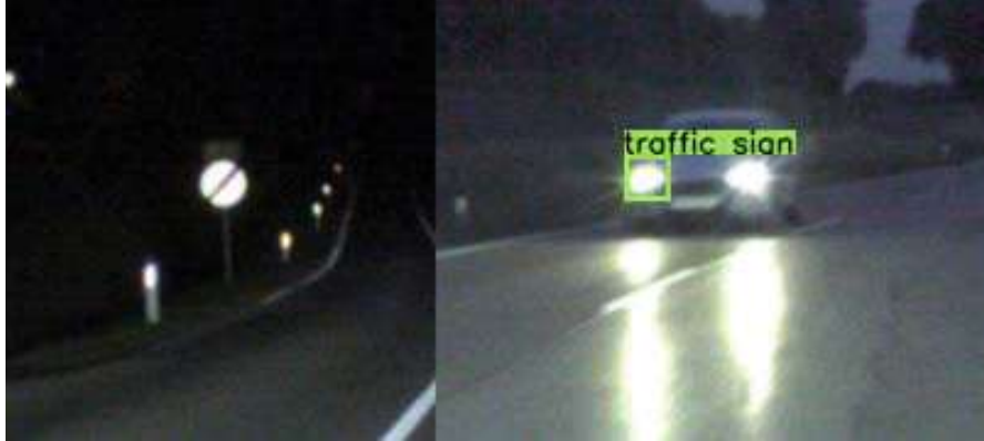
Figure 5.11: The left image shows a traffic sign on the road. The image on the right side shows an oncoming car being falsely labelled as “Traffic Sign”. This image highlights the similarity between a traffic sign at night with the headlights of an oncoming car.
