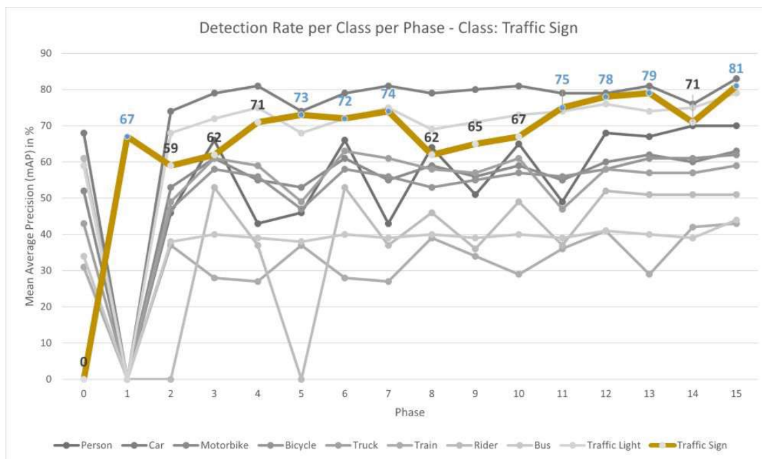
Figure 5.10: Detection results (mAP) in % split by class and phase. The focus of this graph is the class “Traffic Sign”, shown in light brown, with each mAP shown for each phase. The blue highlighted data points shows where the GTSRD dataset was added to the training dataset.
