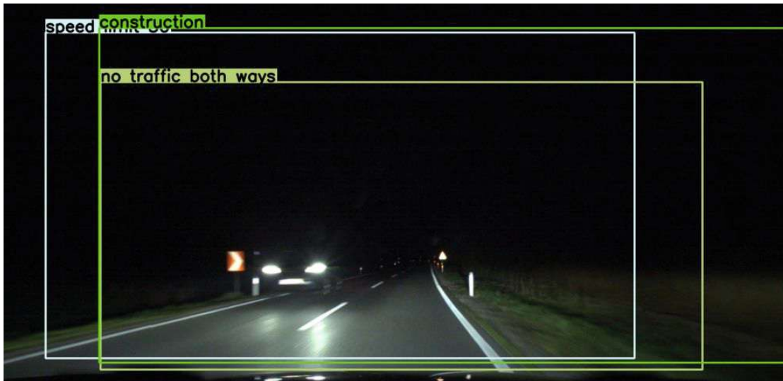
Figure 5.16: Example of false positive object detection for different traffic sign classes. The whole image was labelled as different street signs, while the street signs and car in the image were not found.
