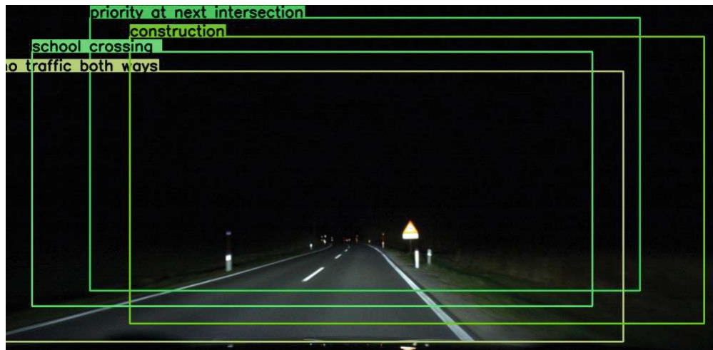
Figure 4.9: Example result of training the network with individual classes for traffic signs, tested on the CVL test dataset. Several false positives were found, with a multitude of street signs being detected.
