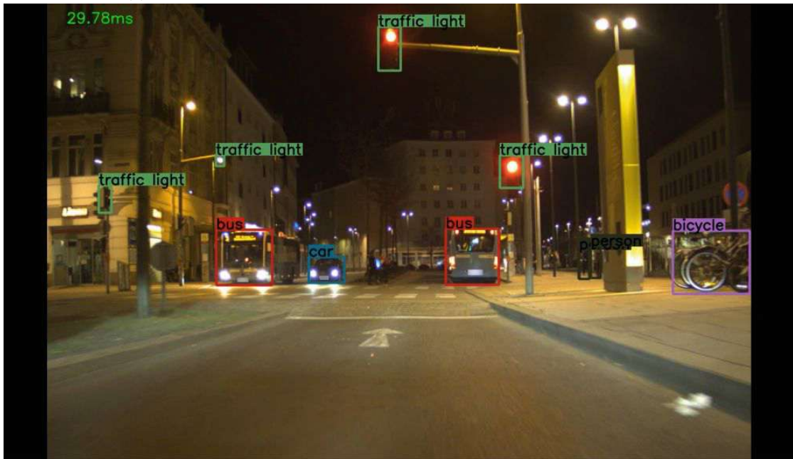
(b) A second frame, taken from the same test video as Subfigure (a). This image was taken a few frames after the one depicted in Subfigure (a), whereby the person next to the bus and one traffic light were not detected.
