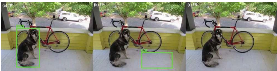
Figure 2.19: Examples for (a) True Positive (TP): the network correctly predicts that an object (in this case, a “Dog”) was found. Subfigure (b) shows a False Positive (FP): The network predicts a positive find for an object that is not actually there (in this case a “Cat”). Finally, (c) shows a False Negative (FN): There are objects in the image that should be detected, but the network fails to find them.
