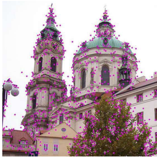
Figure 2.4: Visualization of SIFT feature points found in an image, after difference of Gaussians has been applied. Source: [sif]
