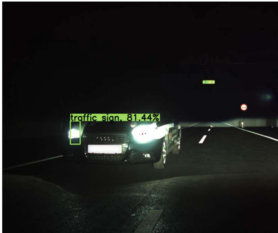
Figure 5.21: Image showing a car with one of the front headlights being detected as a traffic sign with 81.44% accuracy.
