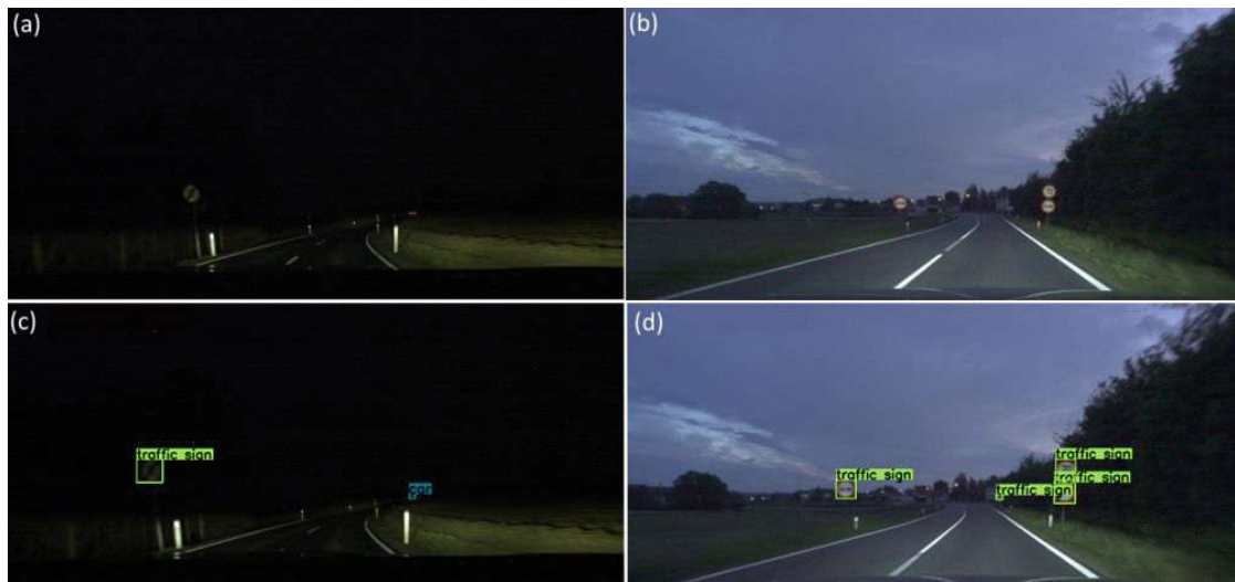
Figure 5.13: Examples of object detection results for different images. Subfigure (a) and (b) were the result of “phase 0”, while Subfigure (c) and (d) were the results of “phase 15”. While no objects are detected in Subfigure (a) and (b), all objects are detected in Subfigures (c) and (d).
