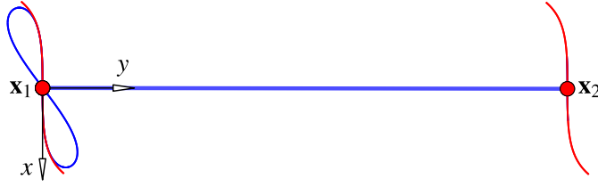
Fig. 4. Reduction of Stachel's double-Watt mechanism to a two-point guidance problem.
