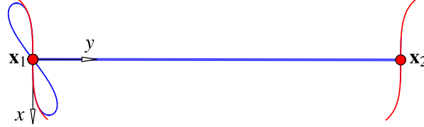
Fig. 2. Reduction of the double-Watt mechanism of Connelly and Servatius to a two-point guidance problem.
