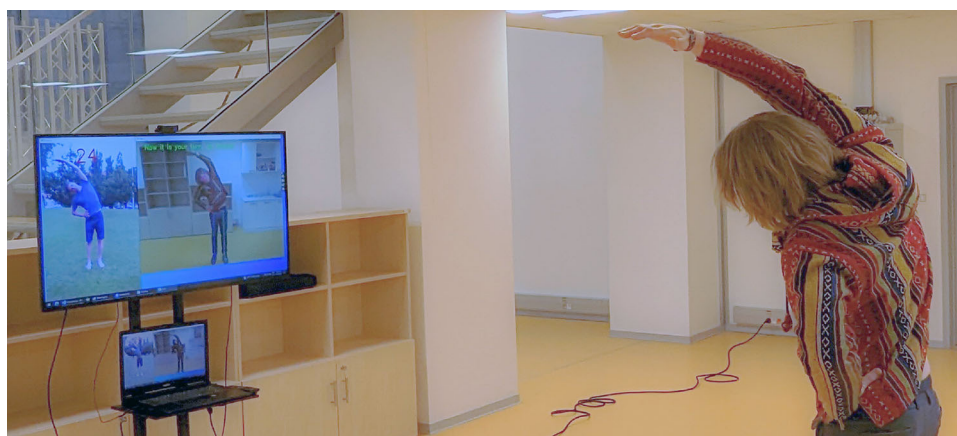
Fig. 1 The OffiStretch system provides guidance for stretching exercises in form of multimodal pre-recorded instructions and real-time visual feedback on a simulated virtual mirror. With this research, we aim to enhance users' motivation to perform physical exercises, help to ensure correct posture for an optimal outcome, and support the automatic analysis of user performance
