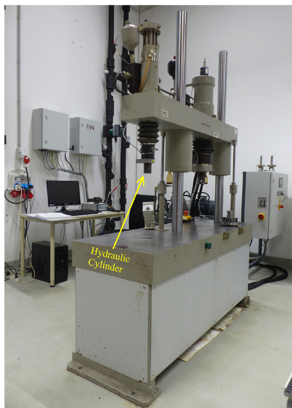
FIGURE 2 Servohydraulic testing machine used for the cube movement experiments.
