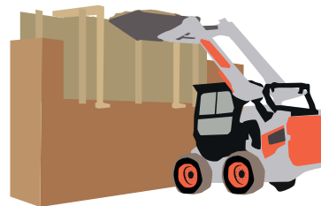
Fig.63: Soil Mixture Being Transported in the Formwork
