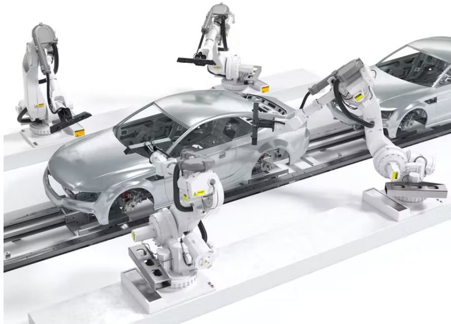
Figure 2.2: Collaboration of several ABIS II for car body surface inspection directly at the assembly line. The optical 3D sensors are mounted to the IRs, which allows to perform inspection tasks within few seconds with resolutions down to 10\ \mu\text{m} [31].
