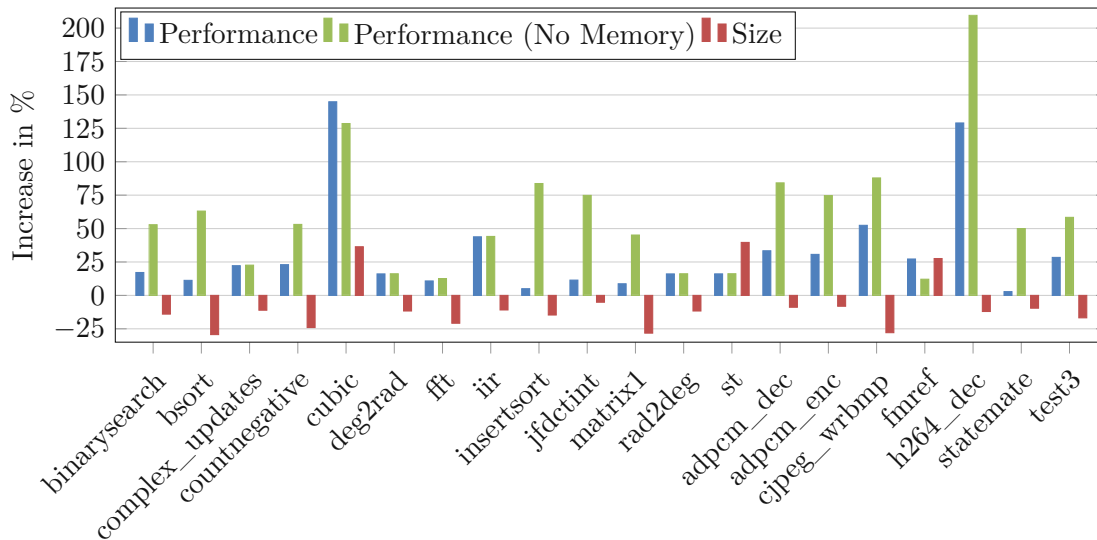
Figure 1.3: Cumulative performance and code size increase of enabling all techniques and optimizations covered in this dissertation.
