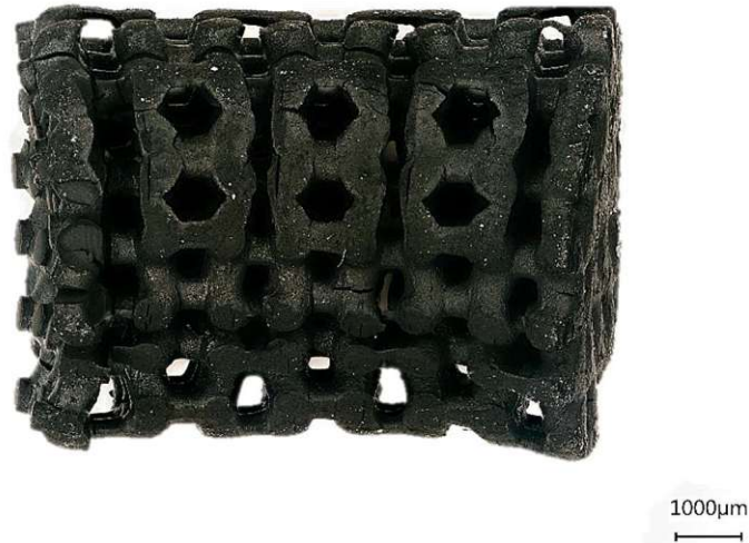
Figure 15: Polymer-derived SiOC ceramic printed with the Photon printer and pyrolyzed at 700 °C in the shape of a complex gyroid. The sample was printed with the Photon printer with an exposure time of 15 sec and a layer thickness of 25 μm per layer.
