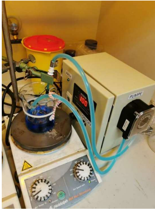
Figure 11: Setup for the adsorption experiment. A methylene blue solution is pumped away from the beaker, through the sample, and back into the beaker. The flow rate is set via the pump controller (grey).
