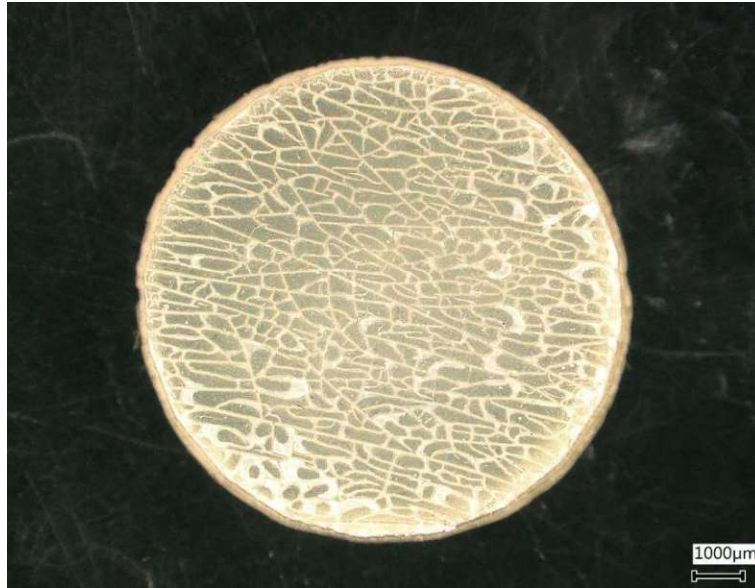
Figure 25: 100 wt.-% PSO2 printed with the Photon printer (with an exposure time of 8 seconds per layer and a layer thickness of 25 \mu\text{m} per layer) and room temperature dried in the shape of a simple cylinder from the top covered with cracks.
