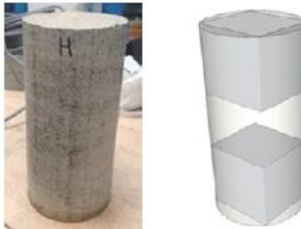
Figure 7: Location of cube sample to be machined in the cylinder (A. Youssef.et.al., 2015)
