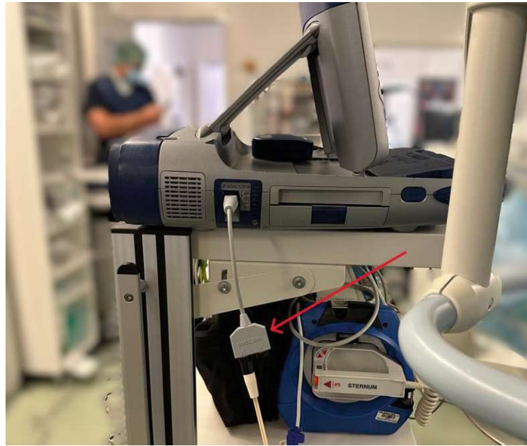
FIGURE 2.1: Medtronic CareLink Programmer: Testing cable which is connected to the patient and EP Tracer
