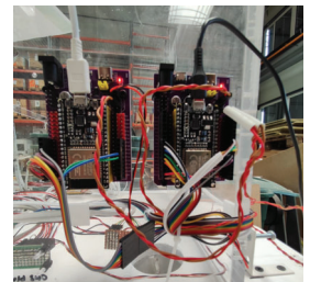
Fig. 3: Digital Twin testbed with from PySIMULTAN generated firmware
